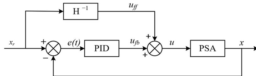
Figure 12. Block diagram of compound control.
