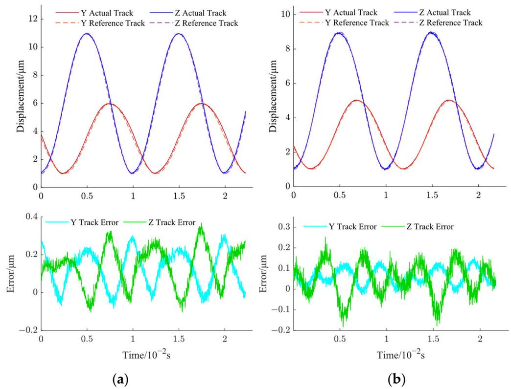
Figure 15. Measured vibration displacements in Y- and Z-directions. (a) Case 1 and (b) case 2.
