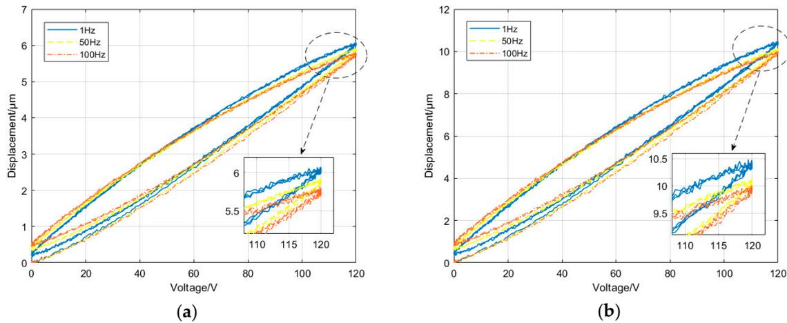
Figure 2. Hysteresis loop curves of the non-resonant EVC device. (a) Y-direction and (b) Z-direction.
