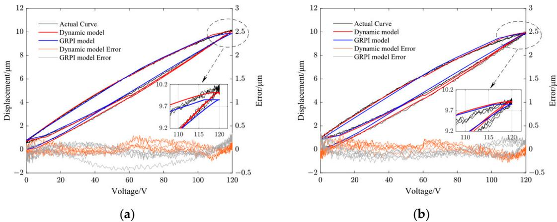
Figure 9. Comparison of dynamic PI model output curve with GRPI model output curve and the model error in Z-direction. (a) 10 Hz and (b) 100 Hz.
