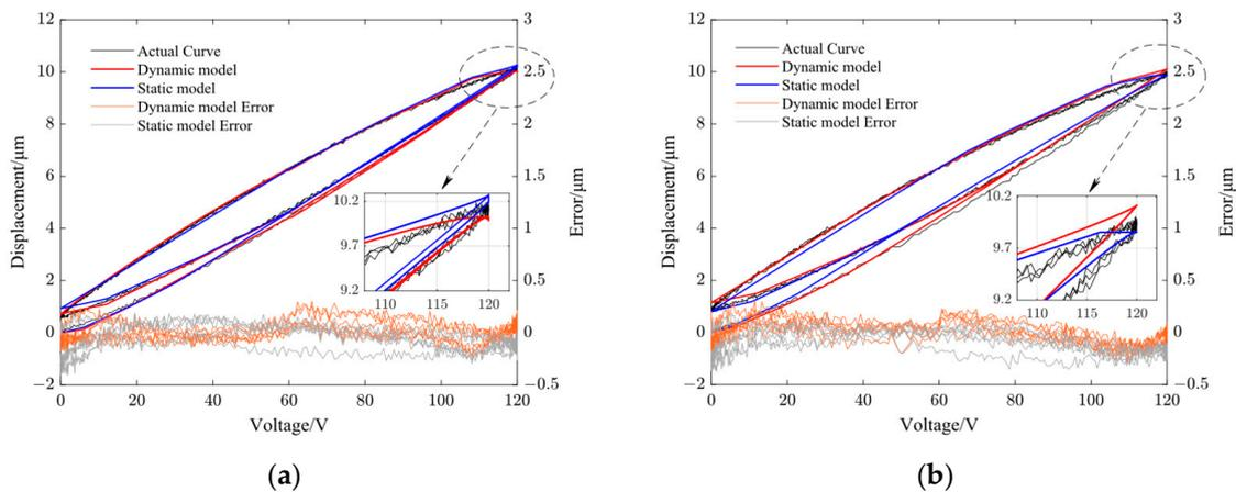
**Figure 11.** Comparison of dynamic PI model output curve with static PI model output curve and the model error in Z-direction. (a) 10 Hz and (b) 100 Hz.
