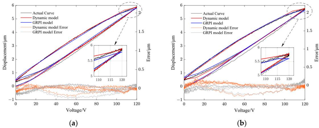
Figure 8. Comparison of dynamic PI model output curve with GRPI model output curve and the model error in Y-direction. (a) 10 Hz and (b) 100 Hz.
