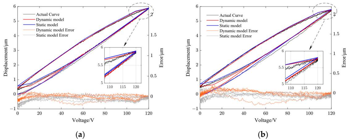
**Figure 10.** Comparison of dynamic PI model output curve with static PI model output curve and the model error in Y-direction. (a) 10 Hz and (b) 100 Hz.
