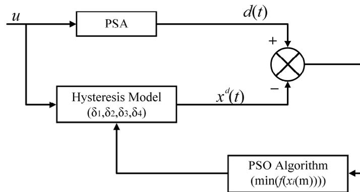
Figure 7. PSO algorithm to identify the dynamical PI model parameters.
