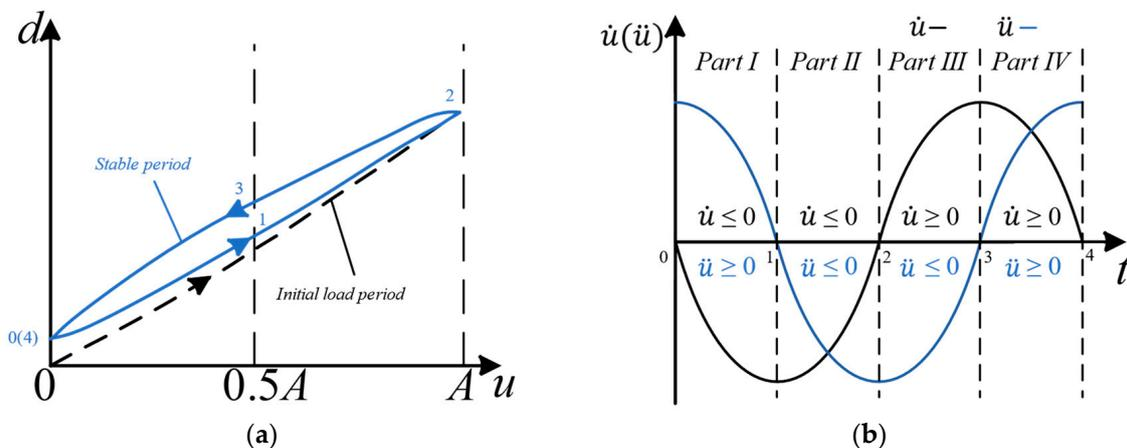
Figure 4. Schematic diagram of hysteresis loop curves. (a) the hysteresis curve of EVC device with a sinusoidal bias voltage; (b) segmentation of hysteresis curve.
