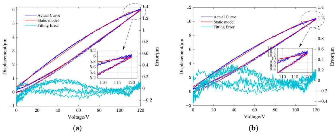
**Figure 5.** Fitting results of the static PI model of the non-resonant EVC device. (a) Y-direction and (b) Z-direction.
