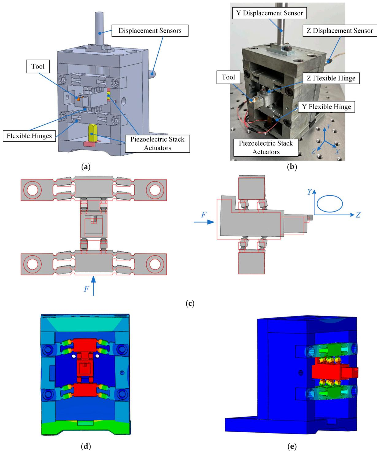
**Figure 1.** The non-resonant EVC device and its working principle. (a) EVC model, (b) EVC device, (c) working principle of EVC device, (d) the first resonant frequency in the Y-direction (482.6 Hz), and (e) the first resonant frequency in the Z-direction (290.7 Hz).
