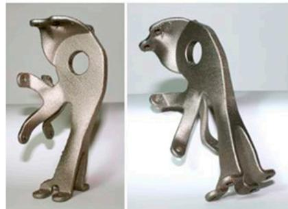
**Figure 8.** Aluminum alloy parts produced by SLM [51].
