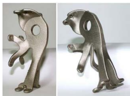
Figure 8. Aluminum alloy parts produced by SLM [52].
