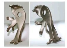
Figure 8. Aluminum alloy parts produced by SLM [51].
