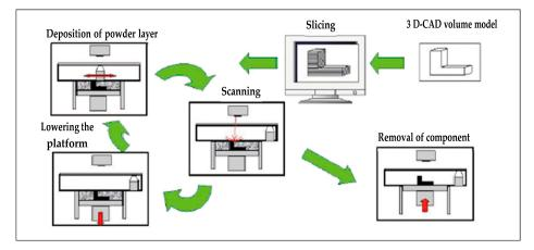
Figure 1. Principle of the SLM process [7].
