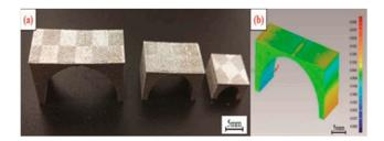
**Figure 10.** 316L Bridge model made by SLM: (**a**) A sample of a bridge-shaped structure; (**b**) the deformation diagram [75].
