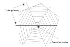
Figure 4. Schematic diagram of spiral fill scanning.
