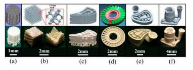
**Figure 11.** Advanced ceramic parts manufactured with SLM [90]: (**a**) porous bioceramic scaffolding; (**b**) photonic crystals; (**c**) hollow turbine blade; (**d**) impeller; (**e**,**f**) investment casting moulds.
