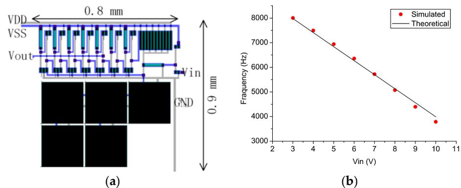
Figure 5. (a) Layout of the proposed VCO, and (b) simulated and theoretical V-f characteristics of the proposed VCO.
