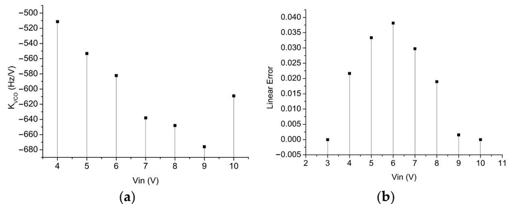
Figure 6. Simulated (a)  $K_{VCO}$  and (b) linear error of the proposed VCO.
