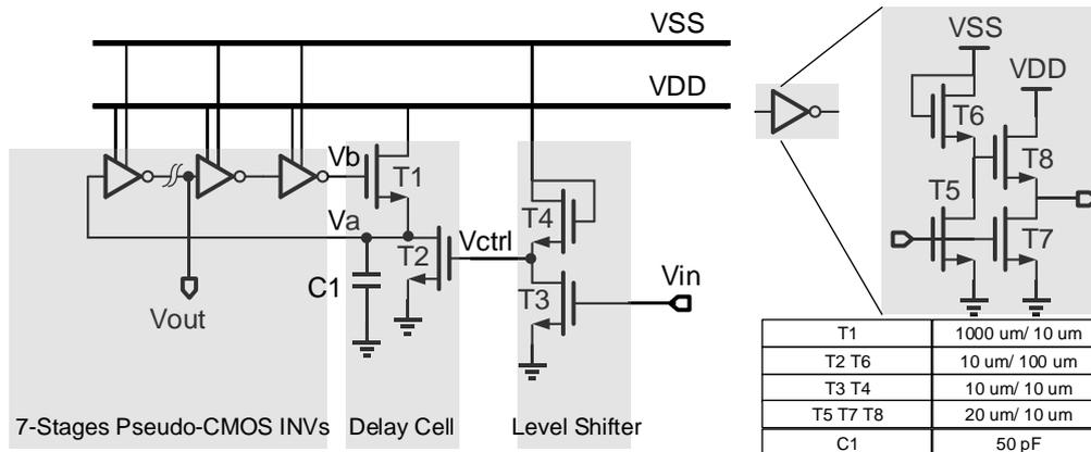
Figure 3. Schematic of the proposed TFT VCO.
