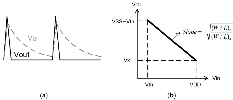
**Figure 4.** (a) Qualitative sketch of the main waveforms of the proposed VCO, and (b) voltage transfer curve of the level shifter.
