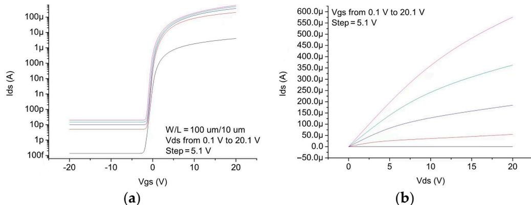
Figure 2. Simulated (a) transfer and (b) output curves of the IZO TFT device.
