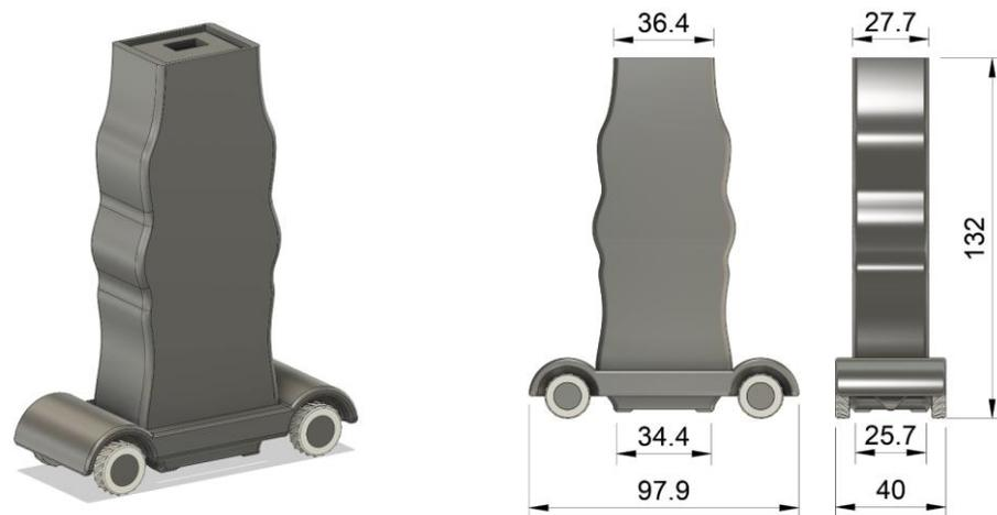
**Figure 13.** Three-dimensionally printed enclosure of the device (dimensions in mm).
