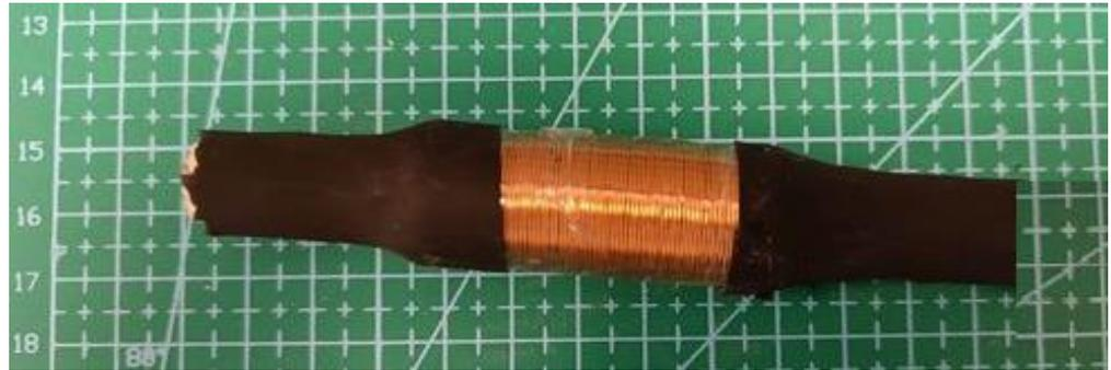
**Figure 5.** A finished microgenerator.
