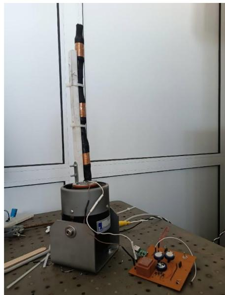
Figure 8. Oscillation generator connected to the power management circuit.
