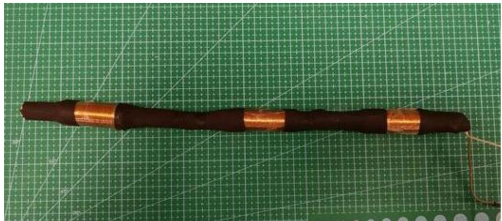
**Figure 6.** Microgenerator system of three generators.
