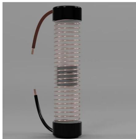
**Figure 3.** Microgenerator with inertial mass inside the coil (3-D rendering).
