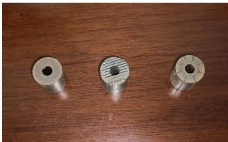
**Figure 5.** Three structures of Terfenol-D rods for experiment.
