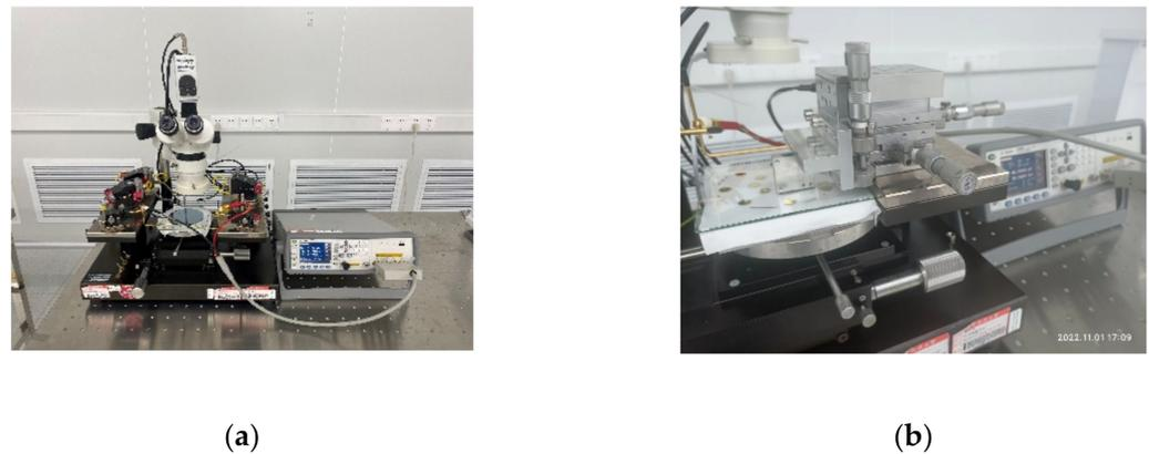
**Figure 7.** Experimental sets, (a) the experimental sets for measuring the surface profile of wafers; (b) the experimental sets for calibrating the capacitive spacing transducer.
