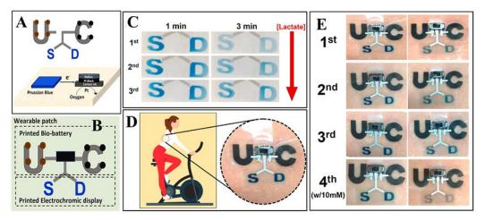
**Figure 2.** Sweat-powered wearable electrochromic biosensor for lactate monitoring. **(A)** Design and working principle of the wearable sweat sensor. **(B)** Different parts of the sensor i.e., printed biobattery and electrochromic display. **(C)** Change in color of the electrochromic display after addition
