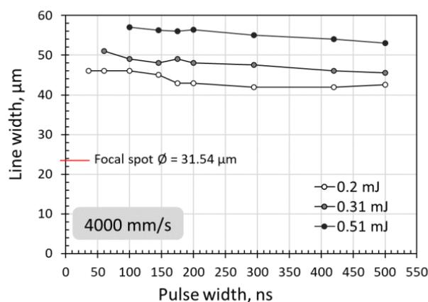
**Figure 12.** Scanning line width versus pulse energy fluence, showing that there are no significant changes with pulse width at energy fluences far beyond the ablation threshold.
