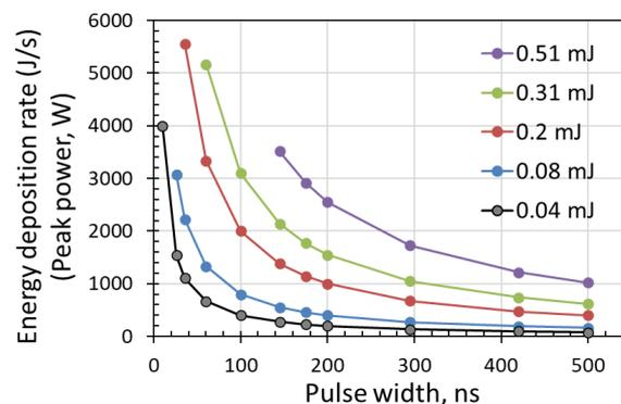
**Figure 4.** The pulse energy deposition rate in terms of laser peak power versus pulse width at different pulse energies.
