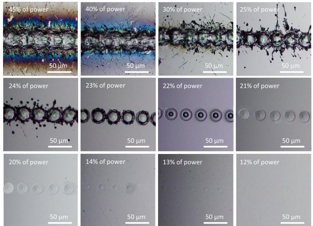
**Figure 5.** Surface morphologies showing surface ablation or melting under various power levels at 100 kHz and 4000 mm/s scanning speed.
