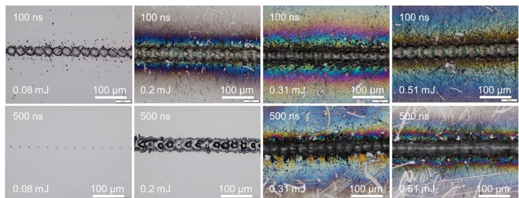
Figure 11. Surface morphologies showing a stronger edge thermal effect and more debris along the scanning line at increasing pulse energy fluence at 400 mm/s scanning speed.
