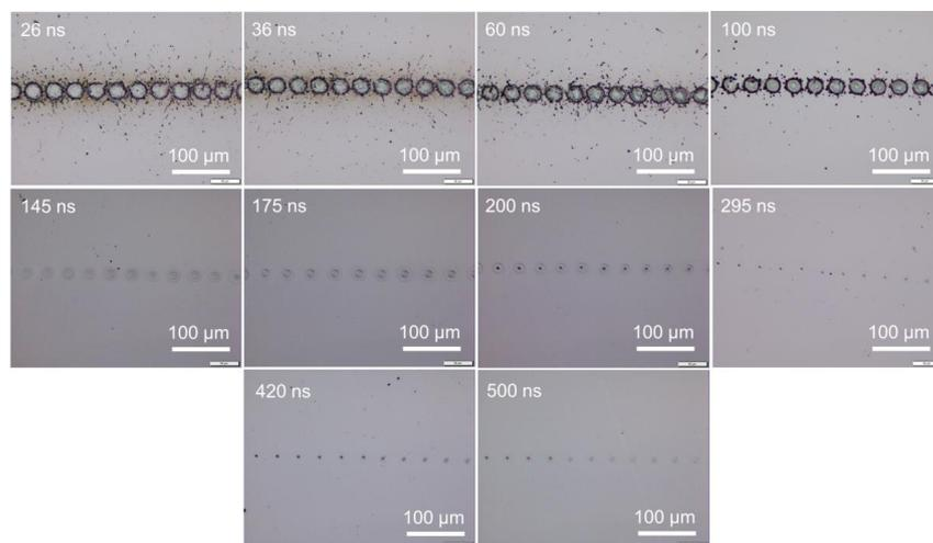
**Figure 3.** Optical images of irradiated silicon surfaces with 0.08 mJ pulse energy (10.24 J/cm<sup>2</sup>) at a scanning speed of 5000 mm/s.
