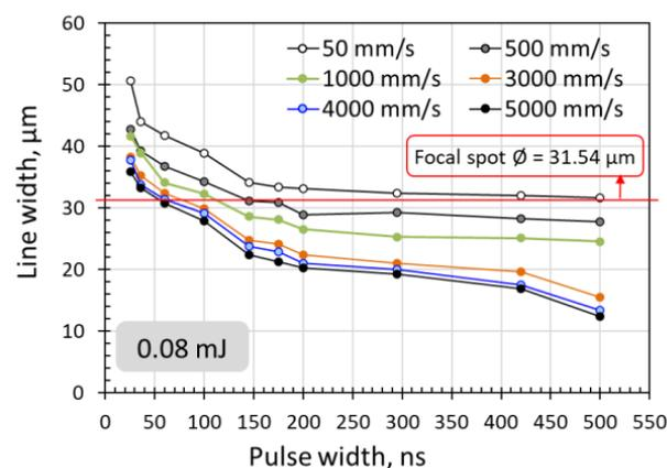
**Figure 9.** Reduction of scanning line width with increasing pulse width for 0.08 mJ pulse energy ( $10.24 \text{ J/cm}^2$ ) at various scanning speeds.
