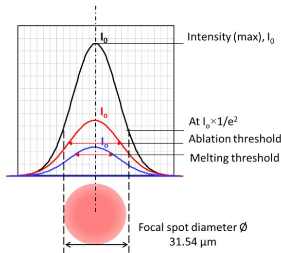
Figure 10. Increase in spot size with pulse energy. Different power percentage  $p$  gives different maximum energy intensity  $I_0$ .
