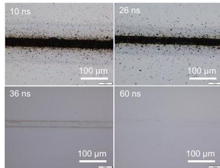
**Figure 1.** Optical images of irradiated silicon surfaces with 0.04 mJ in pulse energy (5.12 J/cm<sup>2</sup>) at a scanning speed of 50 mm/s.
