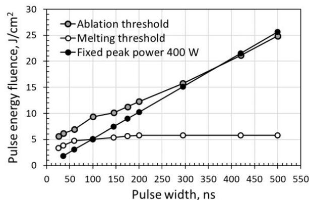
**Figure 6.** Variation of surface ablation and melting thresholds with pulse width.
