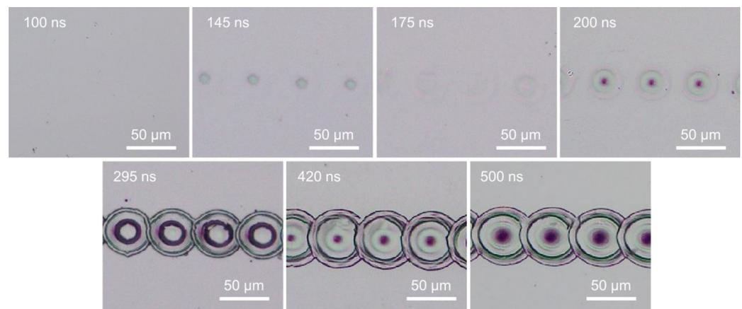
**Figure 7.** Surface morphologies showing surface melting with increasing pulse width at 4000 mm/s scanning speed.
