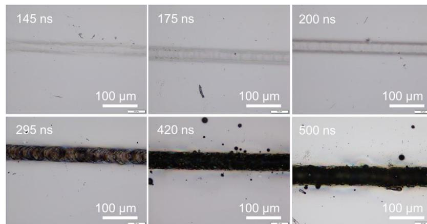
**Figure 8.** Surface morphologies showing enhanced surface melting with increasing pulse width at 50 mm/s scanning speed.
