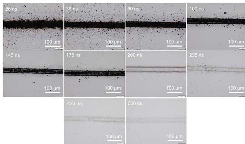
**Figure 2.** Optical images of irradiated silicon surfaces with 0.08 mJ pulse energy (10.24 J/cm<sup>2</sup>) at a scanning speed of 50 mm/s.
