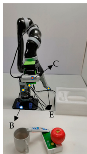
Figure 9. Coordinate System Declaration. Where B is the base coordinate system, E is the End Actuator Coordinate System, C is the camera coordinate system.
