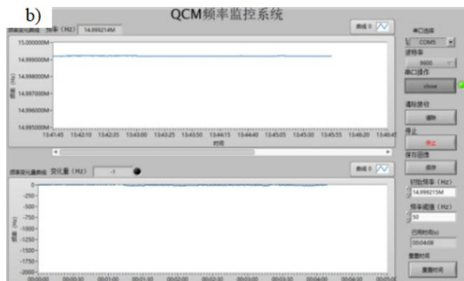
**Figure 9.** (a) Interface for testing RNA virus positive samples (The title of the diagram indicates: QCM frequency acquisition system.); (b) interface for testing negative RNA virus samples (The title of the diagram indicates: QCM frequency acquisition system.).
