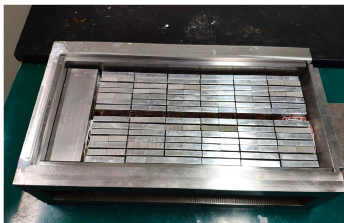
Figure 8. The transducer array was put in the filling mould.
