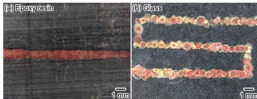
**Figure 8.** A demonstration of copper patterning. (a,b) Metal deposition by scanning the bubble injector in a I and S shape.
