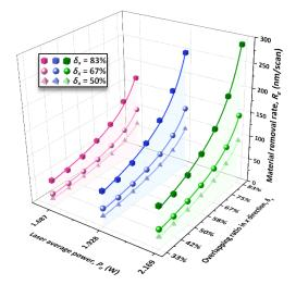
**Figure 11.** The material removal rate ( $R_e$ ) versus the overlapping ratios of the laser spot at different average laser powers.
