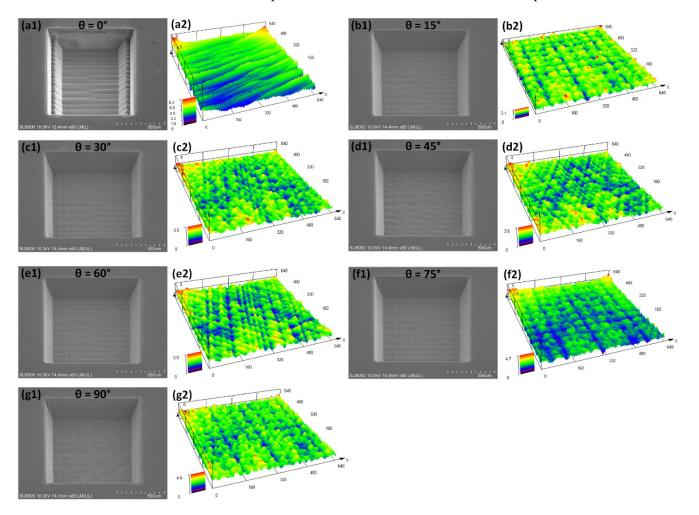
**Figure 12.** (**a1–g1**) SEM images and (**a2–g2**) LSCM measurements of the square trenches machined only by changing the hatch rotation angle ( $\theta$ ) from 0° to 90° at the laser average power of 2.169 W, the scanning speed of 1000 mm/s, and the hatch spacings of 5 µm.
