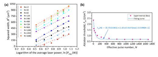
**Figure 5.** (a) The widths of all the ablated microgrooves versus the average laser powers under different effective pulse numbers. (b) The relationship between effective pulse number and ablation threshold.
