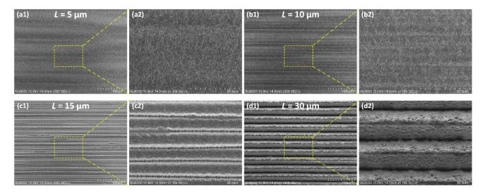
**Figure 9.** The bottom surface topography of deep trenches machined using different hatch spacings of (**a1**) 5  $\mu$ m, (**b1**) 10  $\mu$ m, (**c1**) 15  $\mu$ m and (**d1**) 30  $\mu$ m and their enlarged views of (**a2–d2**) at the average laser power of 2.169 W and the scanning speed of 1000 mm/s.
