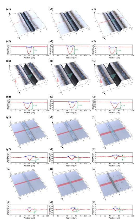
**Figure 4.** LSCM images of ablated microgrooves (N = 240) at different average laser powers of (**a1**) 1.687 W, (**b1**) 1.928 W, (**c1**) 2.169 W, (**d1**) 2.410 W, (**e1**) 2.651 W, and (**f1**) 2.892 W and their profile data in (**a2–f2**). LSCM images of ablated microgrooves (N = 12) at different average laser powers of (**g1**) 1.687 W, (**h1**) 1.928 W, (**i1**) 2.169 W, (**j1**) 2.410 W, (**k1**) 2.651 W, and (**l1**) 2.892 W and their profile data in (**g2–l2**).
