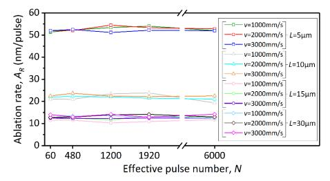
**Figure 8.** The ablation rate ( $A_R$ ) of the trenches versus the effective pulse number (N) at different hatch spacings (L).
