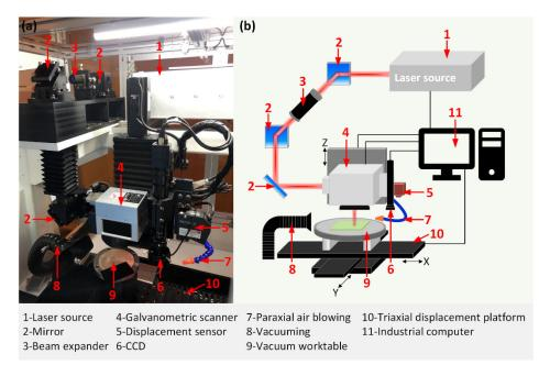
Figure 1. (a) Picture and (b) schematic of the laser workstation.
