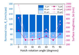
**Figure 13.** The material removal rate ( $R_e$ ) and surface roughness (*Sa*) versus the hatch rotation angles at different hatch spacings of 5, 10, and 15  $\mu$ m.
