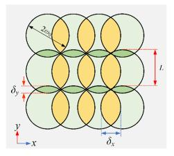
**Figure 7.** Illustration of overlapping ratios of the laser spot in x ( $\delta_x$ ) and y ( $\delta_y$ ) directions.
