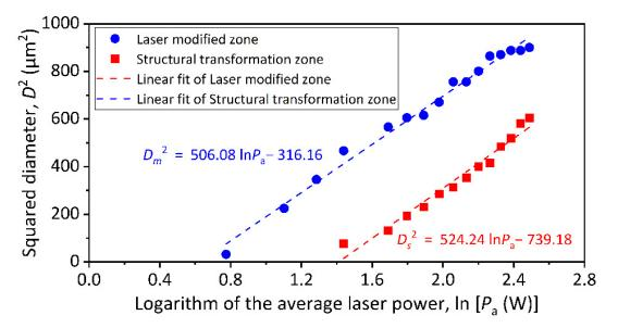
Figure 3. Fitting function curves of the squared diameters and the average laser powers.
