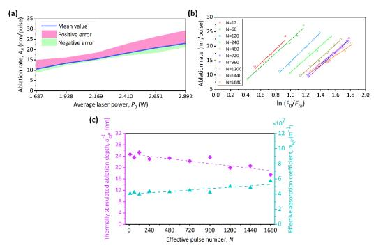
**Figure 6.** (a) The ablation rate of the microgrooves versus the average laser power. (b) The ablation rate versus  $\ln(F_0/F_{th})$  for different effective pulse numbers. (c) Results of the thermally stimulated ablation depth and the effective absorption coefficient for different effective pulse numbers.
