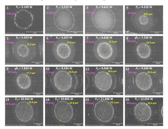
images of ablated microgrooves processed by the effective pulse number of 240 are shown in Figure 4(a1-f1). Their profile data in Figure 4(a2-f2).
