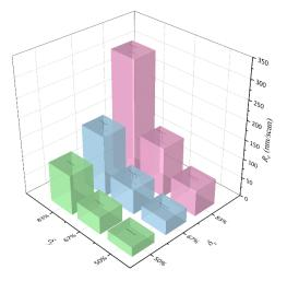
**Figure 10.** The material removal rate ( $R_e$ ) versus the overlapping ratios of the laser spot in x ( $\delta_x$ ) and y ( $\delta_y$ ) directions at the average laser power of 2.169 W.
