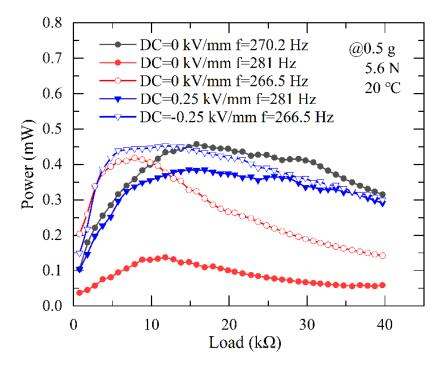
Figure 5. The output power tuning performance of the PEH under different DC electric fields.
