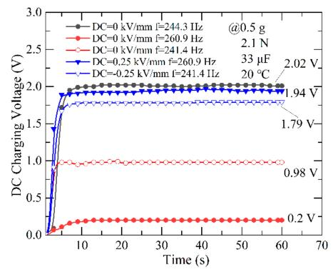
Figure 6. The charging response tuning performance of the PEH under different DC electric fields.
