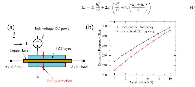
where EI represents the bending stiffness, which can be given by
