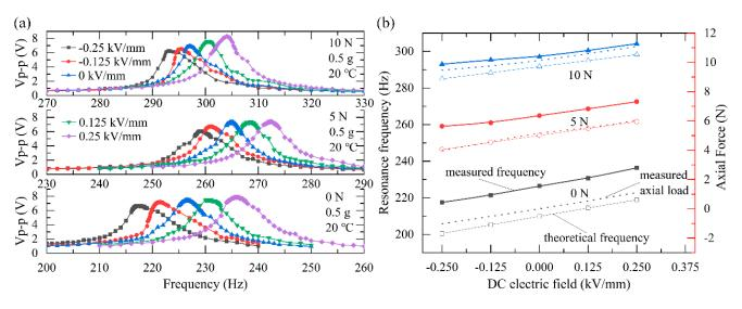
**Figure 3.** (a) The output voltage as a function of frequency under different DC electric fields and axial preload; (b) The measured resonance frequency, the measured axial preload, and the theoretical resonance frequency under different DC electric fields and different preloads.
