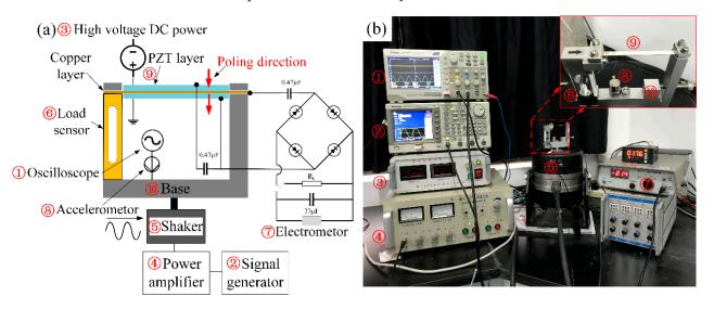
Figure 2. (a) Illustration of the measurement setup; (b) Photograph of the experimental setup.
