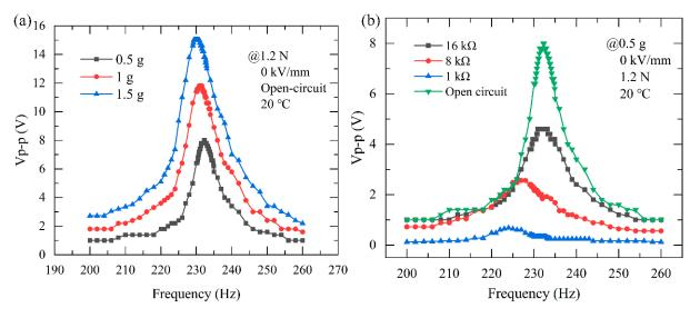
**Figure 4.** The output performance of the PEH. (**a**) Output response voltage as a function of frequency under different acceleration; (**b**) Output response voltage with various load resistances.
