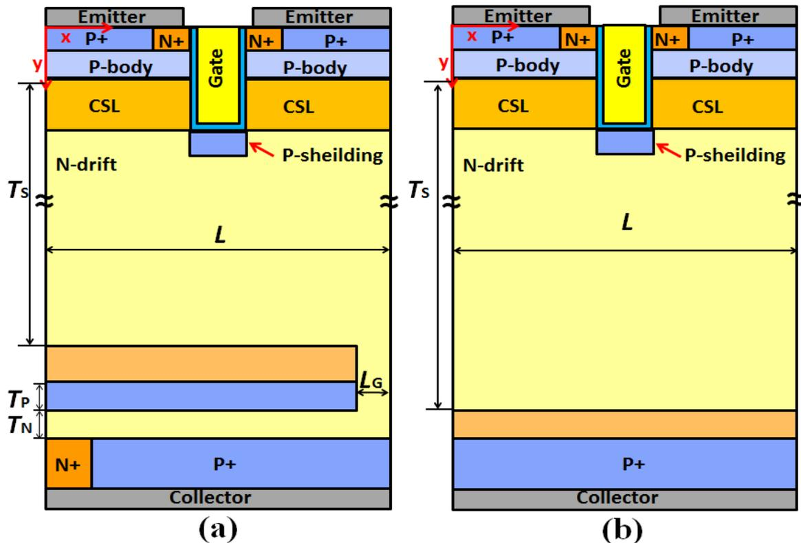
Figure 1. (a) Illustrative cross-sectional diagram of the MP-IGBT, and (b) of the conventional FS-IGBT.
