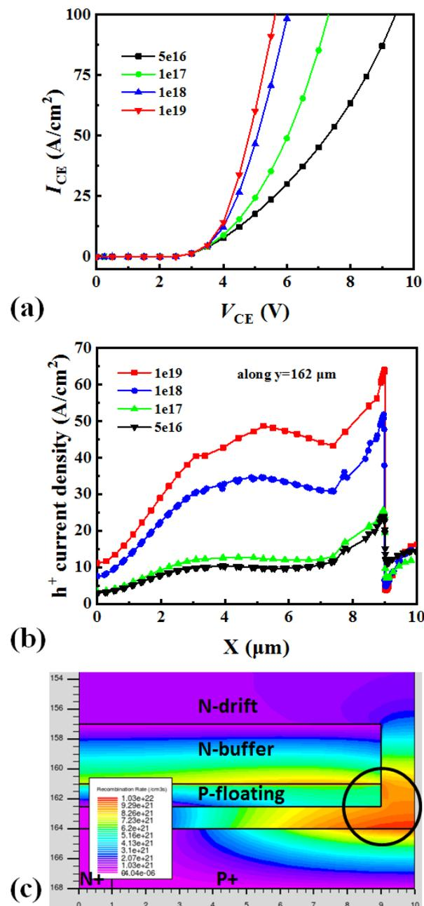
**Figure 9.** (a) Dependence of  $I$ - $V$  curves on the doping concentration of P-floating layer. (b) Dependence of hole current density along  $y = 162 \mu\text{m}$  during on-state. (c) The schematic of recombination rate at the bottom-side structure.
