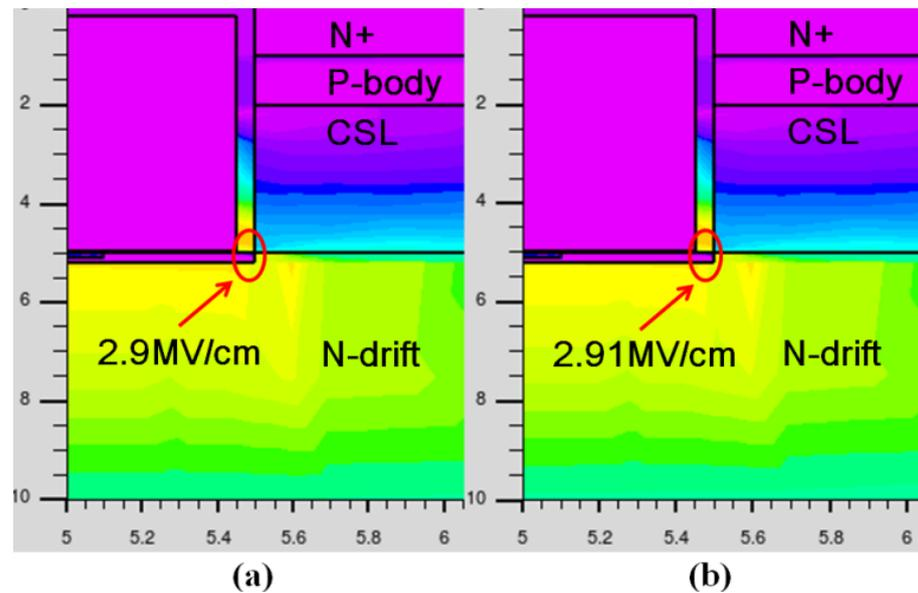
**Figure 4.** Electric field distribution in the top-side structure at  $V_{CE} = 15$  kV. (a) FS-IGBT. (b) MP-IGBT.
