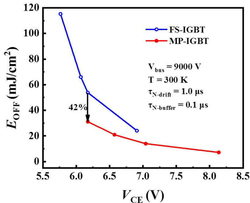
Figure 7.  $E_{OFF}$ - $V_{CE}$  relationships of the MP-IGBT and the FS-IGBT.
