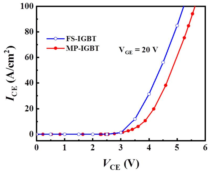
Figure 2. Comparison of the forward  $I$ - $V$  characteristic curves of the MP-IGBT and the FS-IGBT.
