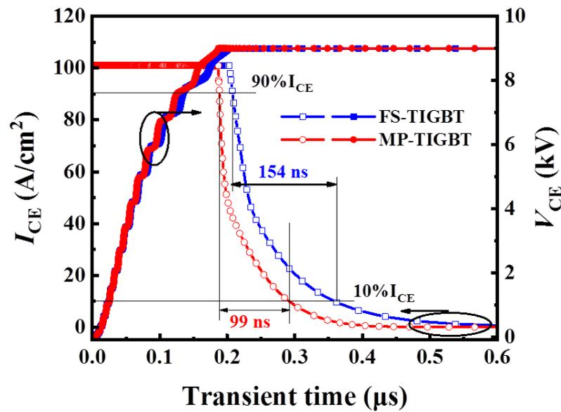
Figure 6. Turn-off voltage and current waveforms of the MP-IGBT and FS-IGBT, respectively.
