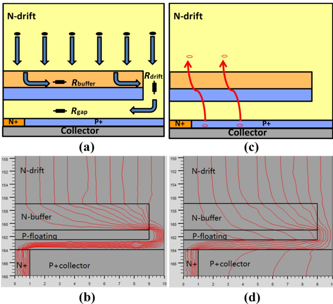
Figure 3. (a) Electron conduction path. (b) Hole conduction path. Current flowlines at the collector side of the MP-IGBT in (c) the unipolar mode and (d) the bipolar mode.
