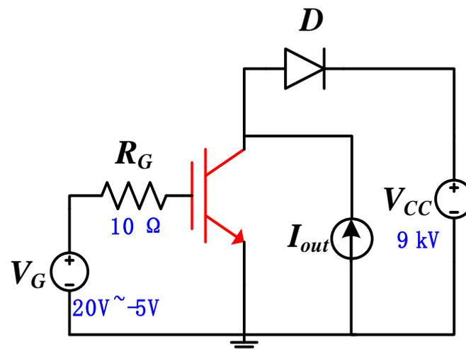
**Figure 5.** Inductive load circuit used in the switching simulations.
