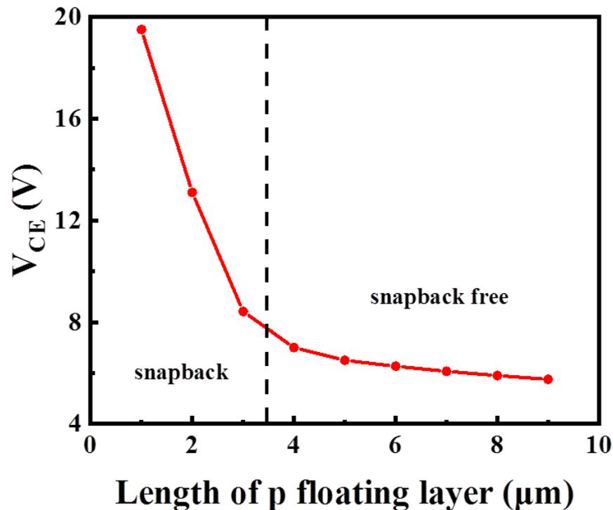
**Figure 8.** Dependence of  $V_{CE}$  on the length of P-floating layer. A longer P-floating layer contributes to lower  $V_{CE}$ .
