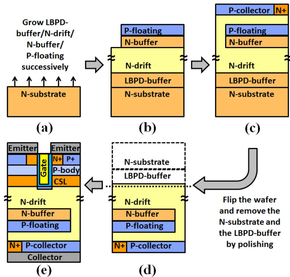
**Figure 10.** (a) The free-standing 4H-SiC N-substrate. (b) Forming LBDP-buffer, N-drift, N-buffer, P-floating. (c) The N-drift, P+, and N+ collector regions are formed by epitaxy and ion implantation. (d) Flip the wafer and remove the N-substrate and the LBDP-buffer by chemical mechanical polishing. (e) The finished MOS structure and electrodes.
