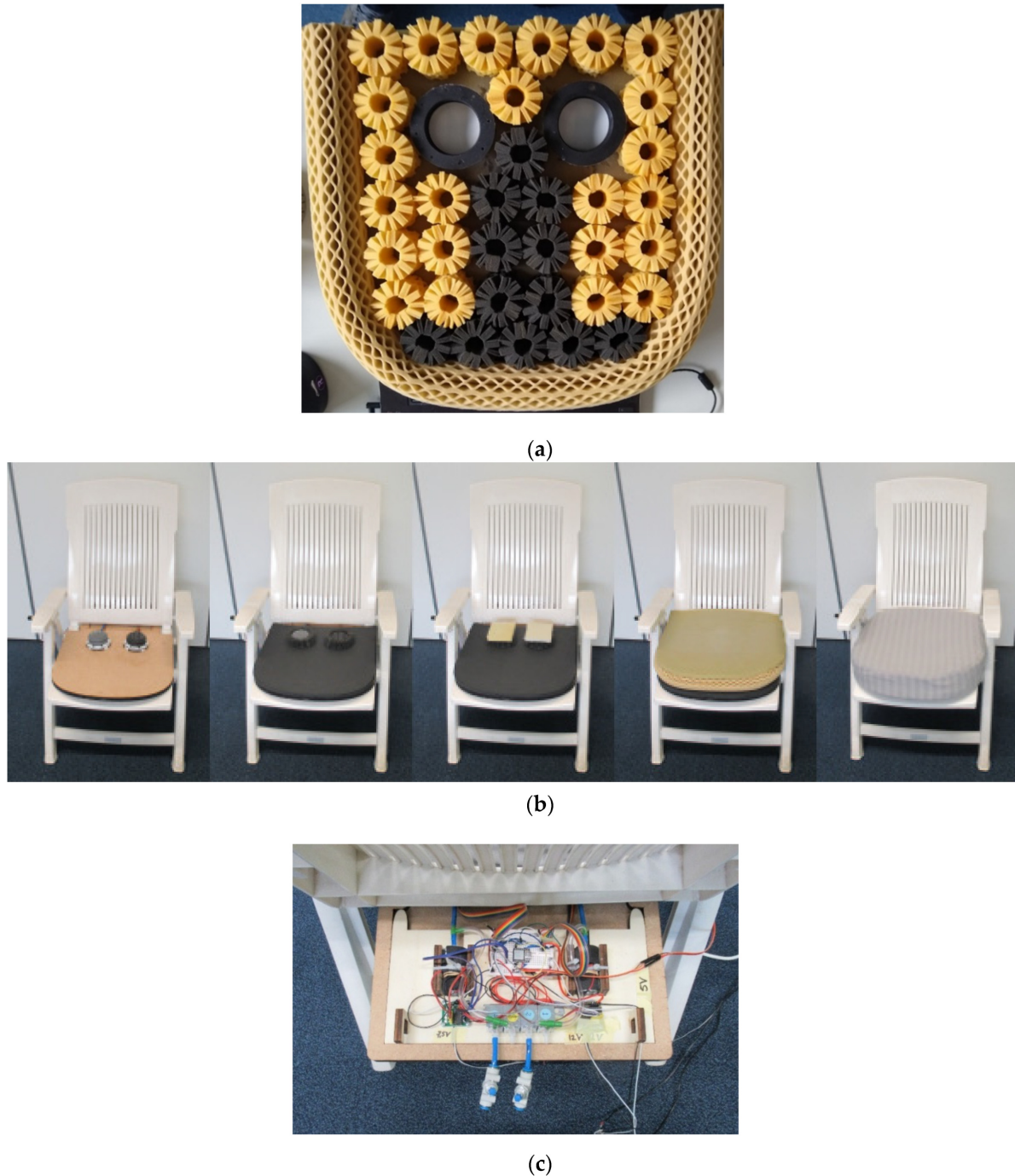
Figure 8. Integration of the soft robotics modules in the chair. (a) Octaspring and the space for the soft robotics module in the cushion (as viewed from underneath); (b) install the soft robotics module to the chair; (c) electronic and pneumatic components positioned under the seat pan.
