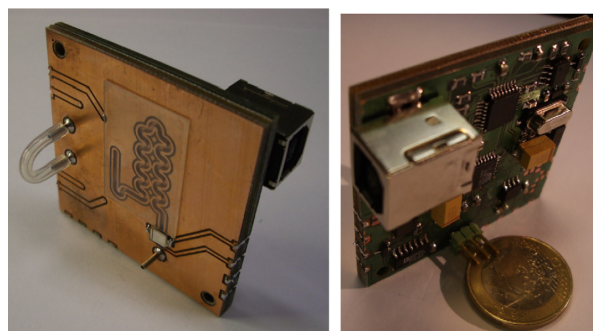
Figure 14. The first lab-on-PCB reported by Stefan Gassmann et al. (reprinted from [11], copyright (2007), with permission from Elsevier).
