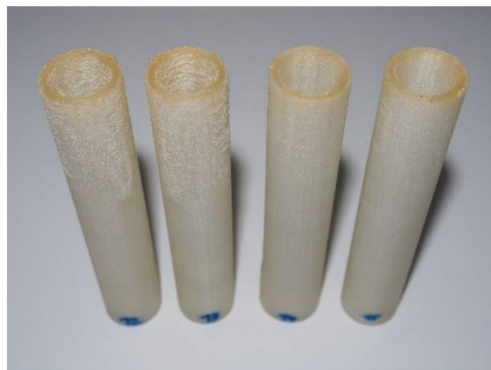
Figure 2. Progress in 3D printed part's quality by using internal support structures from left to right.
