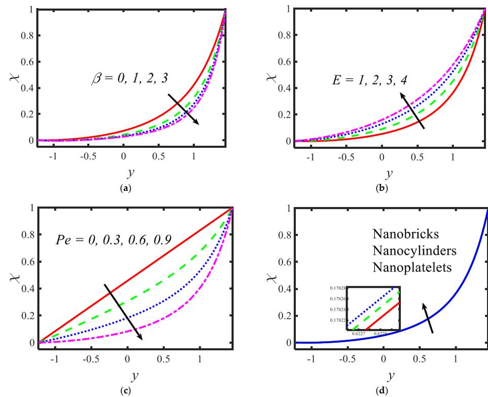
**Figure 6.** Variations in the motile microorganism profile for (a) the temperature ratio parameter, (b) activation energy parameter, (c) Prandtl number and (d) shape factor.
