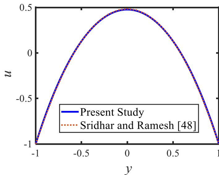
**Figure 8.** Comparison of the velocity profiles of the present study and [51].
