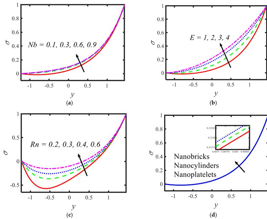
**Figure 5.** Variations in nanoparticle volume fraction profiles for (a) the Brownian motion parameter, (b) activation energy parameter, (c) radiation parameter and (d) the Shape factor.
