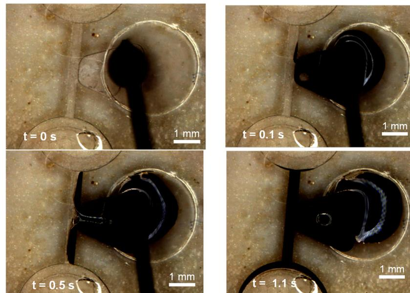
**Figure 4.** Images (with the corresponding time stamps) showing the deposition (using a heated Hamilton syringe) of the molten ferrowax and its subsequent motion due to the action of the capillary forces and the blocking of the fluidic channel.
