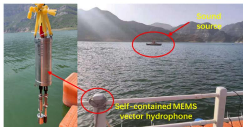
**Figure 17.** Experimental field of ship noise acquisition.
