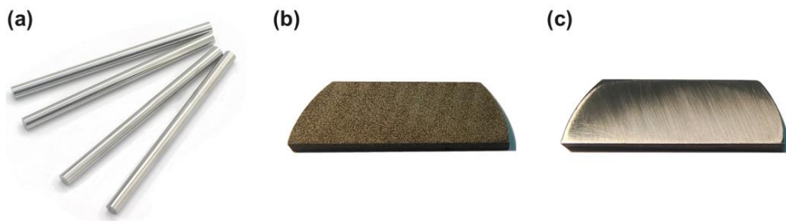
Figure 2. Experimental materials: (a) bar, (b) sheet (after wire cutting), (c) sheet (after grinding).
