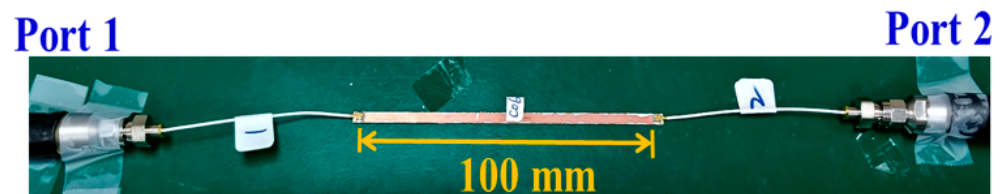
Figure 8. Measurement setup with the test structure and two SMT to SMA cables.
