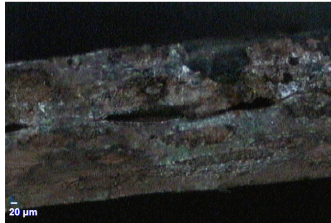
Figure 10. PTFE layers are not properly laminated without a bonding layer.
