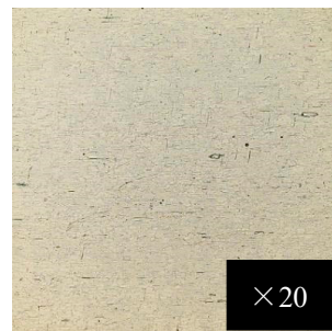
Figure 7. Alumina film on 1060 aluminum substrate observed by confocal microscope.
