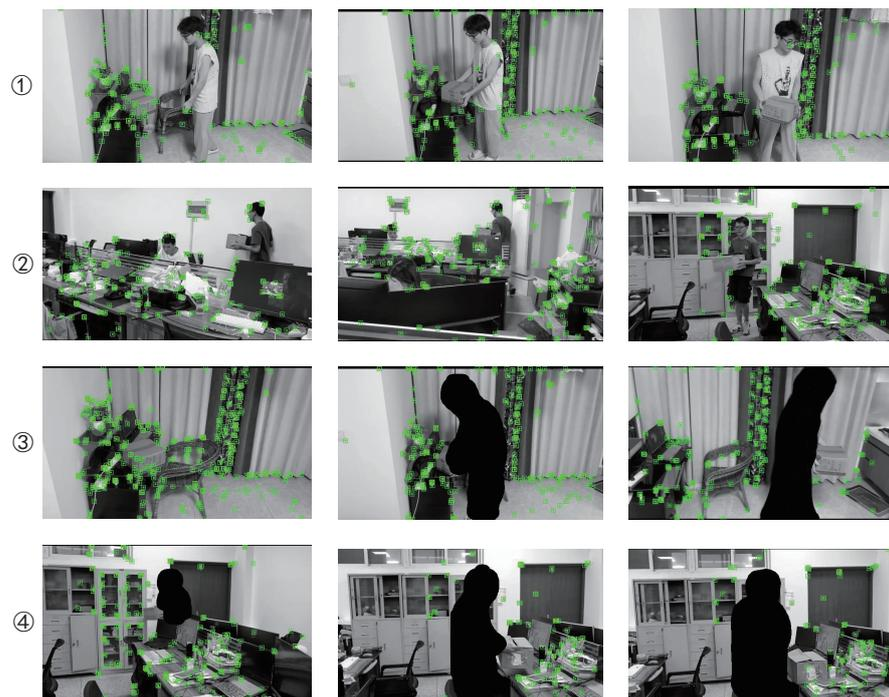
**Figure 12.** Test effect on the real indoor dynamic environment. The pictures in ① and ② lines are test renderings of ORB-SLAM2. The pictures in ③ and ④ lines are test renderings of our method.
