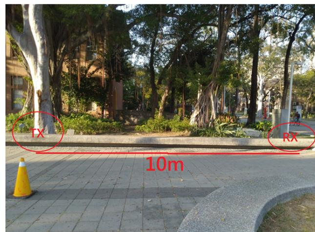
**Figure 16.** SX LoRa-1278 communication experimental environment.
