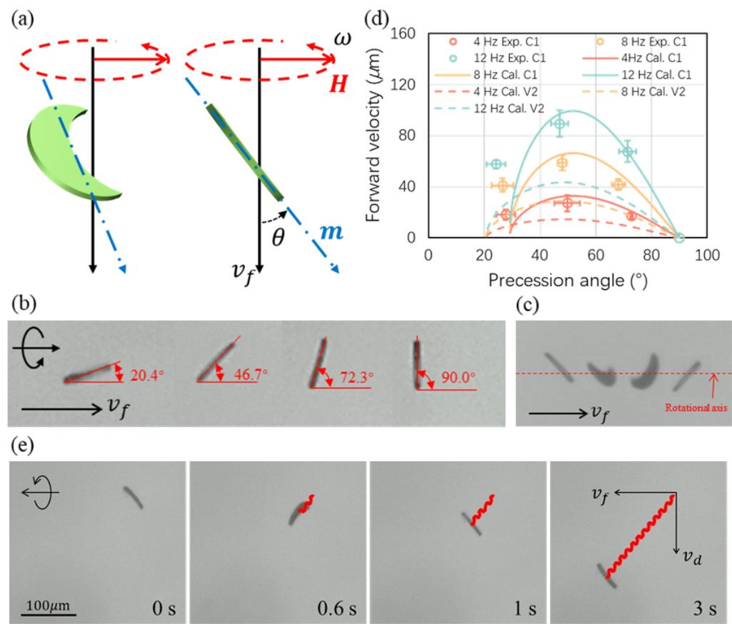
**Figure 4.** (a) Swimming motion of crescent-shaped and V-shaped microswimmer. The angle depicted in the figure is the precession angle; (b) Different swimming motions in experiments; (c) Swimming trajectory of a crescent-shaped microswimmer; (d) The effect of swimming motion or precession angle on forward swimming velocity under the different frequency of the rotational magnetic field; (e) Swimming with precession angle of 45° of a crescent-shaped microswimmer during a half rotation.
