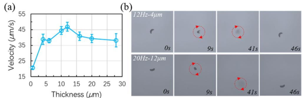
**Figure 6.** (a) Forward swimming velocity of the C1-type microswimmers with different thickness; (b) Out-of-plane (upward) motion of the C1-type microswimmers with different thickness.
