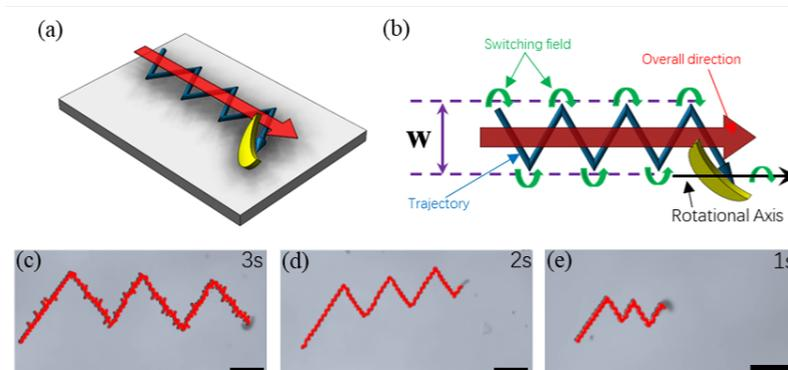
**Figure 7.** (a) Schematic of the zigzag trajectory strategy of a C1 microswimmer achieving overall forward swimming; (b) Schematic of the zigzag trajectory achieved by switching the field direction; (c,d) Zigzag trajectories achieved by a C1 microswimmer with different switching intervals of the magnetic field. Scale bars: 100  $\mu\text{m}$ . (c) 3 s interval. (d) 2 s interval. (e) 1 s interval.
