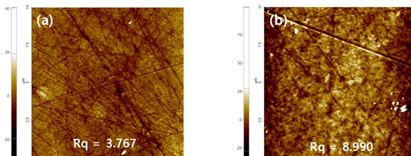
Figure 12. AFM analysis of (a) Ref sample and (b) M0.1N5S1 sample.
