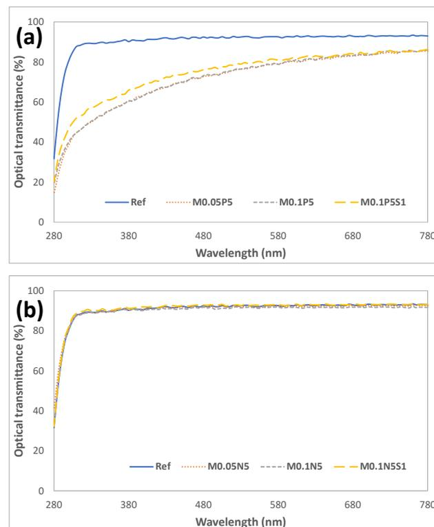
**Figure 3.** Optical transmittance of samples. (a) PVP group; (b) NVP group.
