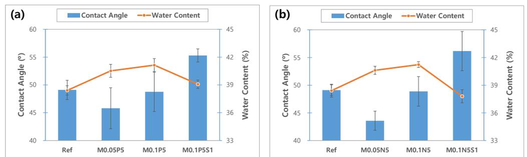
Figure 10. Change of contact angle and water content of samples. (a) PVP group; (b) NVP group.
