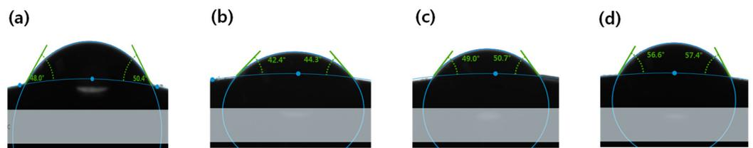
Figure 11. Contact angle image of (a) Ref sample, (b) M0.05N5 sample, (c) M0.1N5 sample, (d) M0.1N5S1 sample.
