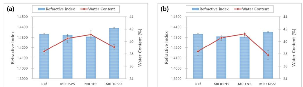
Figure 2. Change of refractive index and water content of samples. (a) PVP group; (b) NVP group.
