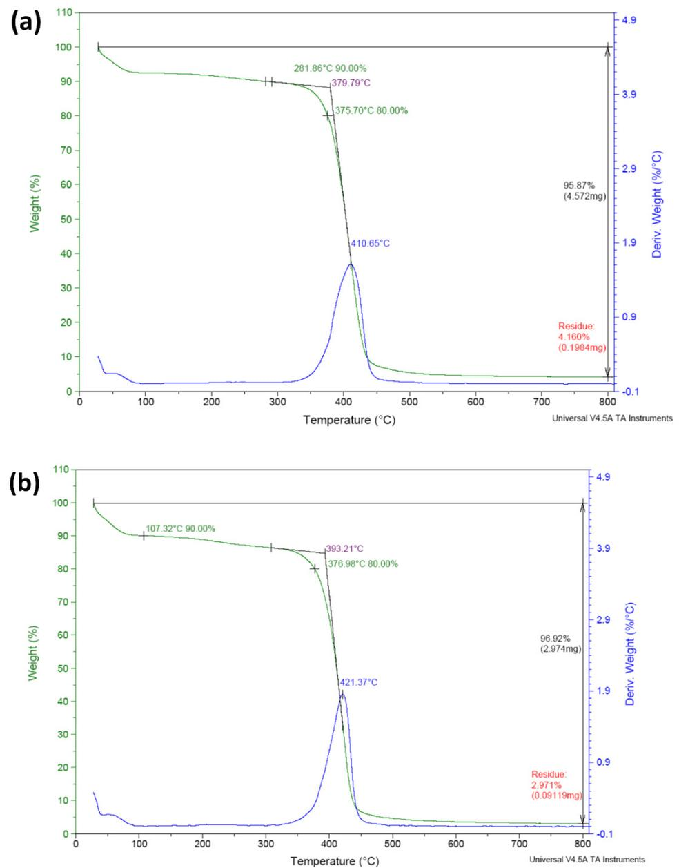
Figure 1. TGA analysis of (a) M0.1N5 sample and (b) M0.1N5S1 sample.
