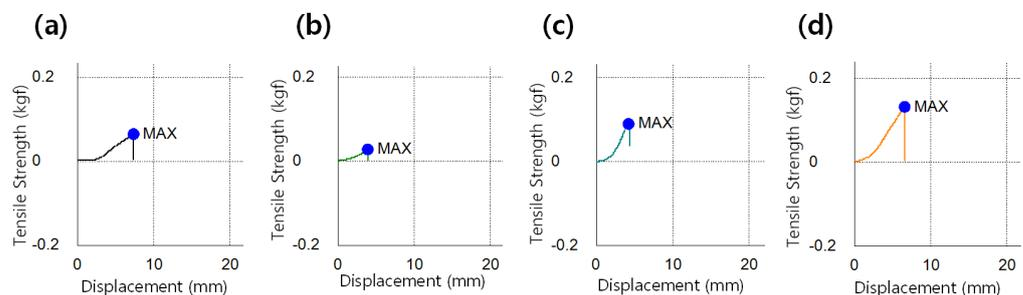
Figure 6. Tensile strength image of (a) Ref sample, (b) M0.05N5 sample, (c) M0.1N5 sample, and (d) M0.1N5S1 sample.
