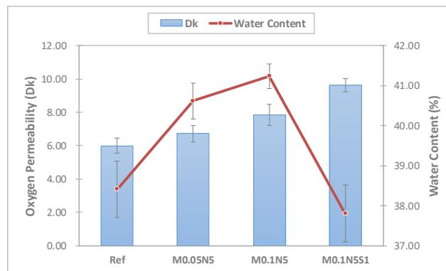
Figure 4. Oxygen permeability and water content of samples.
