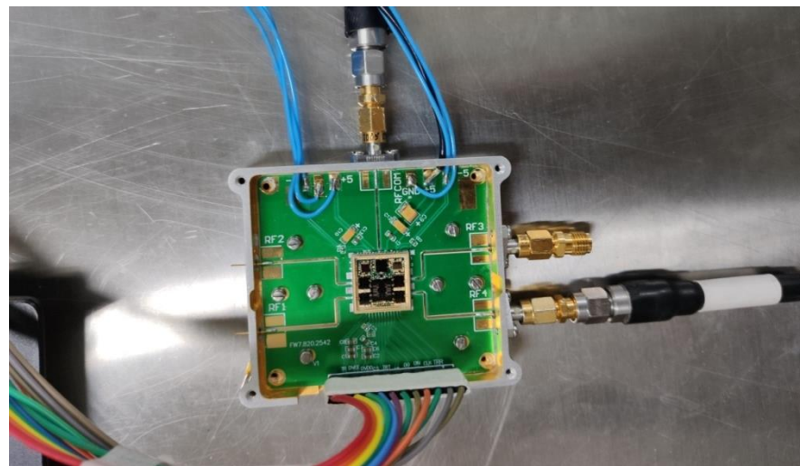
Figure 8. Test fixture of the proposed transceiver SIP.
