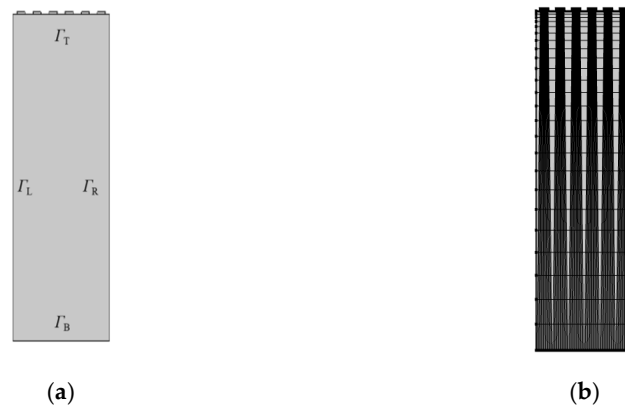
Figure 2. Schematic diagram of structure: (a) schematic diagram of the two-dimensional model; (b) schematic diagram of grid division.
