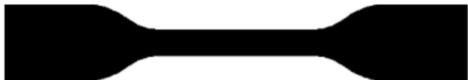
**Figure A3.** BMT template for the 3D inkjet printing of tensile specimens following DIN EN ISO 527-2 type A5 norm.
