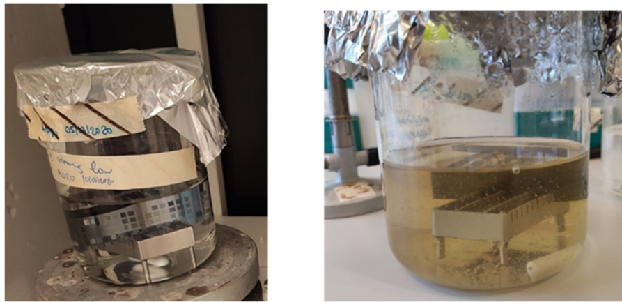
Figure S1: Images of the experimental batch setup consisting of a beaker, a metal rack, the silicon microscope slides on the rack, and the growth media: left, before inoculation; right, after inoculation. [1]
