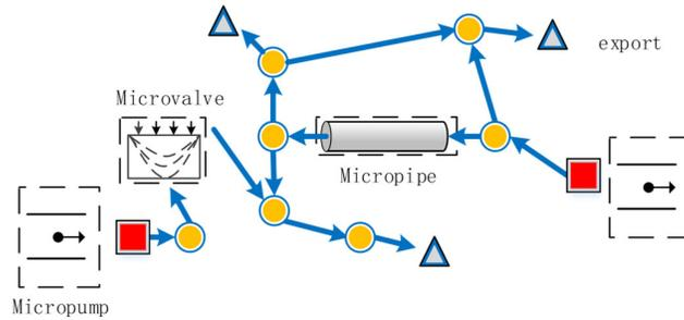
Figure 1. Directed topology model of the microfluidic network.
