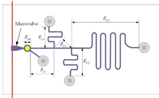
Figure 5. Fluidic resistors of the microfluidic circuit.
