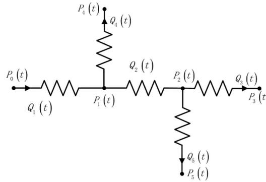
Figure 6. Electrical model of microfluidic platform.
