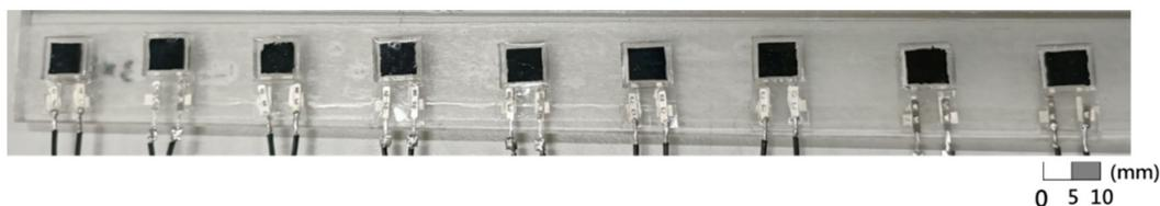
**Figure 14.** Batch production of the 7 wt.% MWCNT doped sensors.
