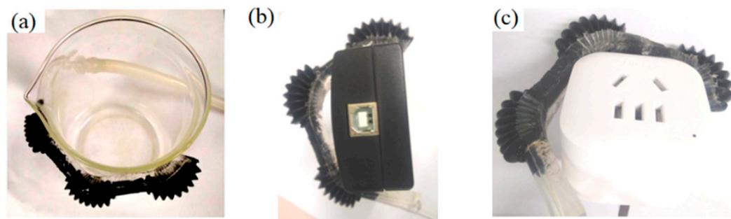
**Figure 9.** Soft robotic digit grasp 3 types of objects: (a) beaker, (b) USB box, and (c) socket.
