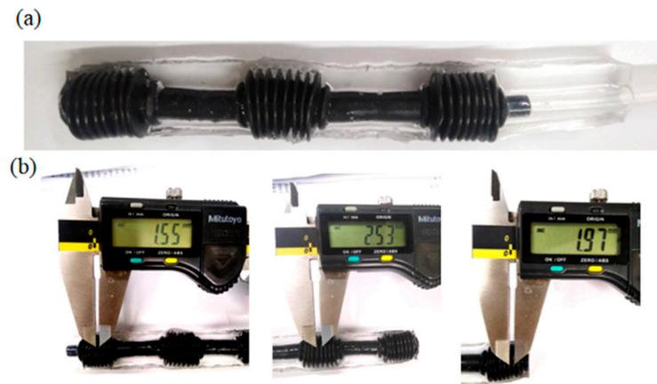
**Figure 4.** Soft robotic finger: (a) a fabricated soft robotic finger with three multi-material pneumatic actuators; (b) different size of each pneumatic actuator.
