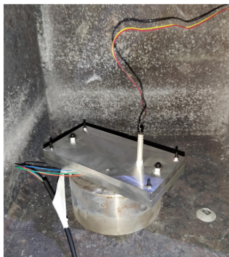
Figure 8. Assembled apparatus for detonation velocity measurement.
