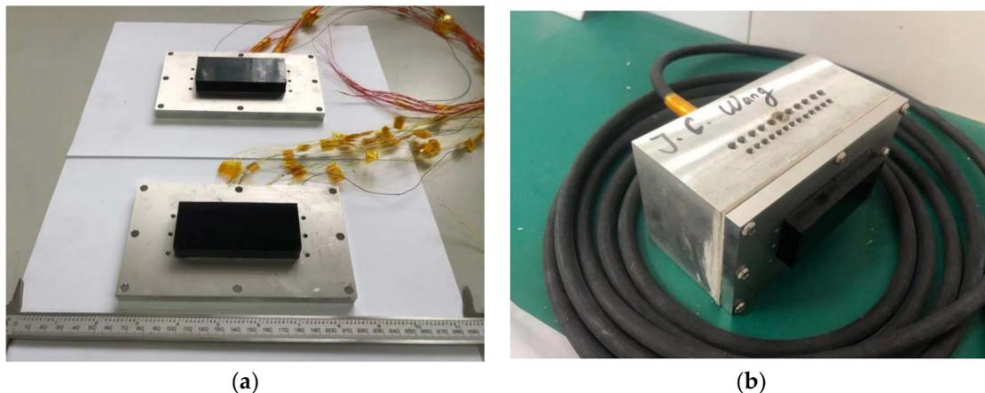
**Figure 10.** Planar array transducer prototypes. (a) Two types of transducer prototypes based on 1–3 piezoelectric composites; (b) Prototype of assembled planar array transducer before test.
