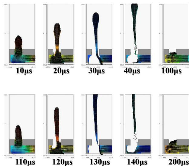
**Figure 5.** Calculate and simulate water in a single-channel jet cavity with a nozzle diameter of  $60\ \mu\text{m}$  and a thickness of  $50\ \mu\text{m}$ , with an operating frequency of  $10\ \text{KHz}$ , in the XZ two-dimensional cross-sectional view, at  $10, 20, 30, 40, 100, 110, 120, 130, 140$  and  $200\ \mu\text{s}$  injection situation.
