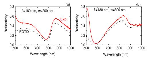
**Figure 6.** Experimental (Exp; red) and calculated (FDTD; dashed) reflectivity spectra of Au nanoprisms with L = 180 nm side length. The thicknesses of the SiO<sub>2</sub> spacer were (**a**) w = 200 nm and (**b**) 300 nm.
