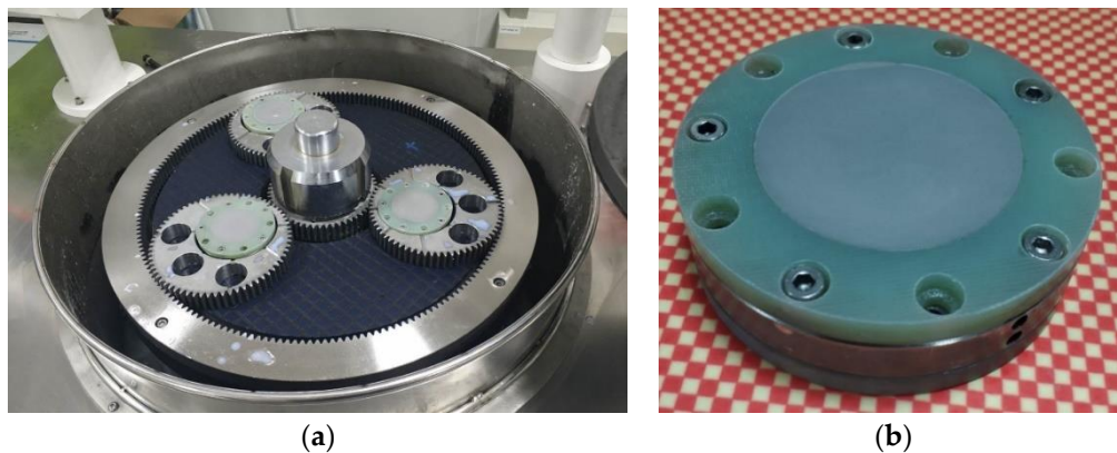
Figure 7. Layer stacked fixture and double-sides polishing equipment: (a) double-sides polishing machine; (b) layer stacked fixture.
