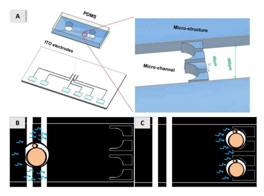
**Figure 1.** Fabrication of the designed DEP microfluidic biochip; (**A**) actual device of size 5 cm  $\times$  3 cm. Bonding of PDMS (microchannel and micro-structures) with the ITO electrode chip. (**B**) The concept of the experiment is that the mouse oocytes and sperm become trapped on the electrodes for about 1 min with the p-DEP. (**C**) Co-incubated 1 h in the micro-structures for natural insemination.
