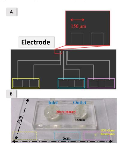
**Figure 2.** (**A**) Three pairs of parallel linear ITO-glass electrodes. (**B**) Actual device (5 cm  $\times$  3 cm). Each gap between the electrodes has width 100 µm; each electrode has width 150 µm.
