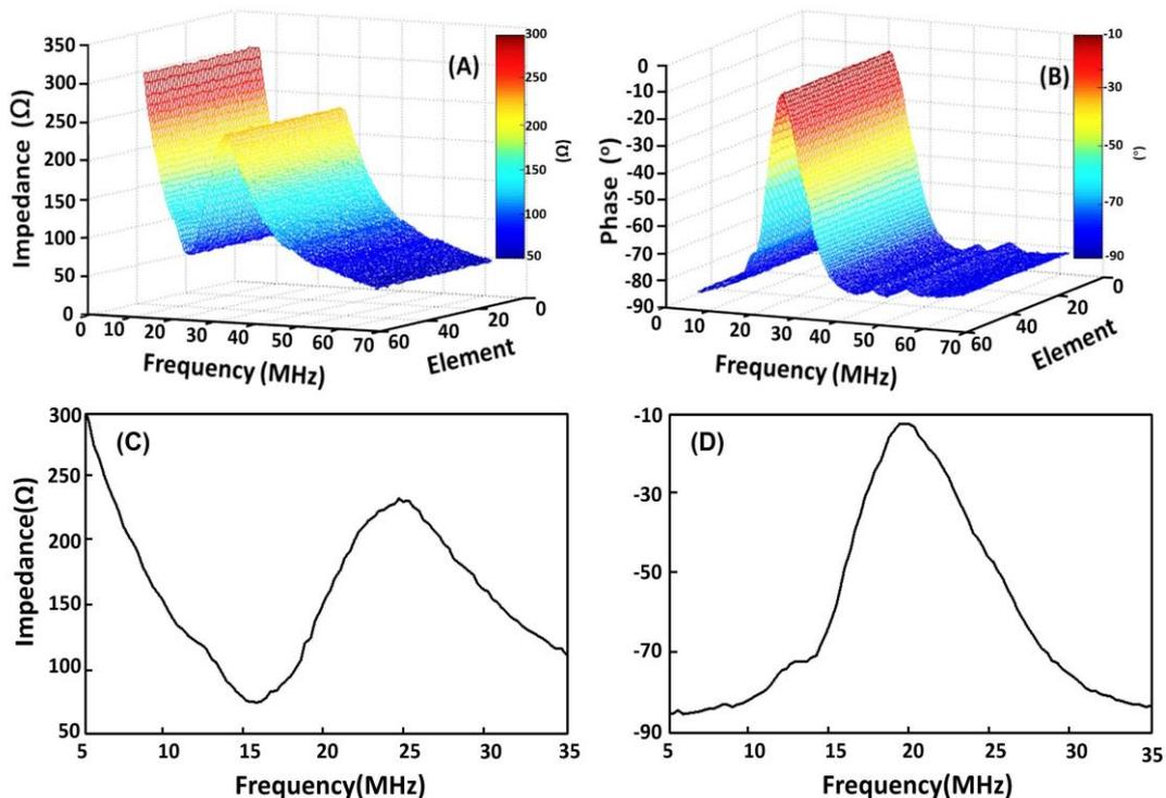
**Figure 4.** (A) Electrical impedance magnitude and (B) phase as a function of frequency for 48 elements. (C) Electrical impedance magnitude and (D) phase as a function of frequency for the 24th element.
