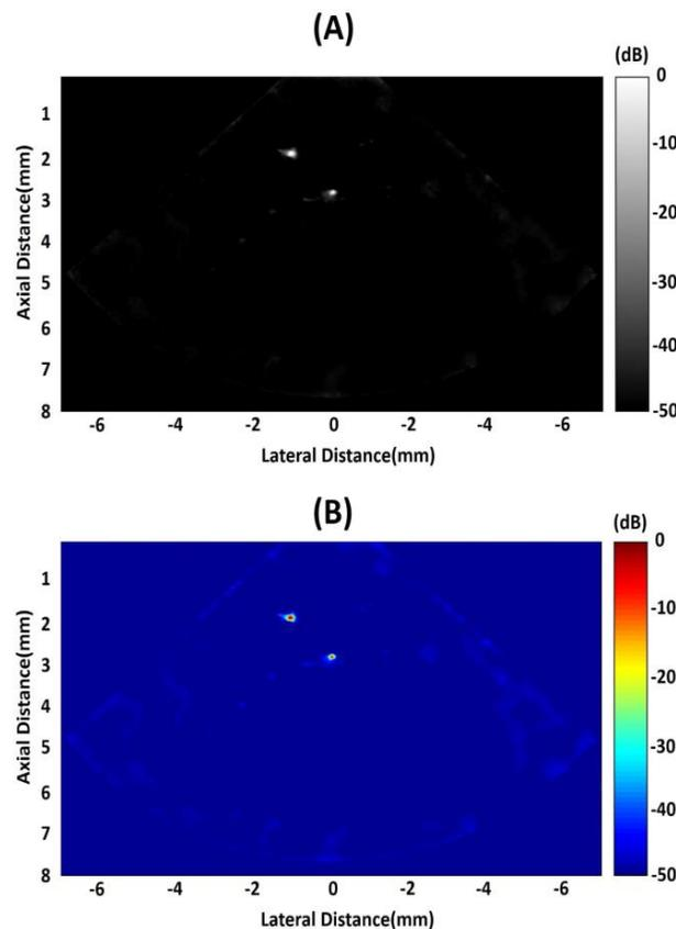
Figure 9. (A) Acquired image of custom-made fine-wire phantom. (B) Pseudo-color image of custom-made fine-wire phantom.
