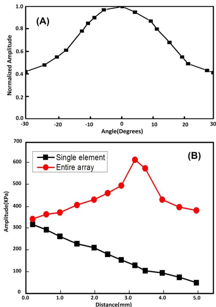
**Figure 6.** (A) Measured one-way azimuthal directivity responses of a representative array element (24th element). (B) The acoustic output in the axial direction of a representative array element (24th element) and the entire array.
