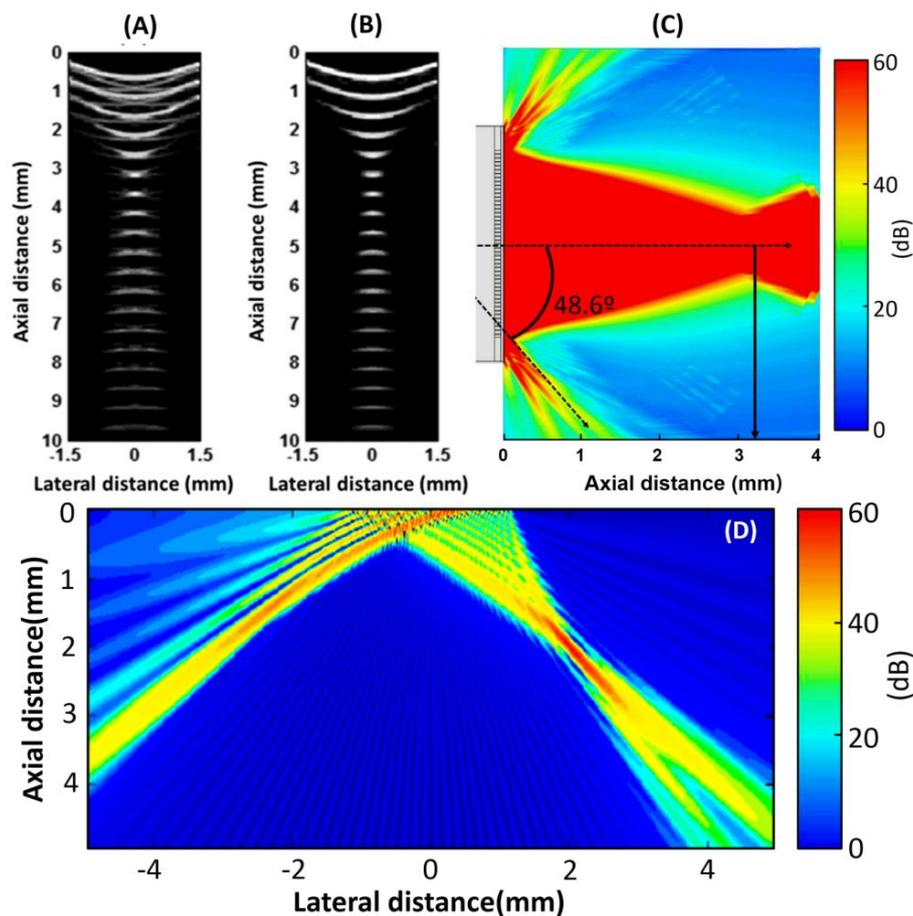
**Figure 7.** Point spread function phantom-imaged (A) without and (B) with apodization. (C) Simulated phased array acoustic pressure of emission mode when the steering angle is  $0^\circ$ . (D) Simulated acoustic beam generated by the 48-element phased array when the steering angle is  $45^\circ$  and the focal distance is 3 mm.
