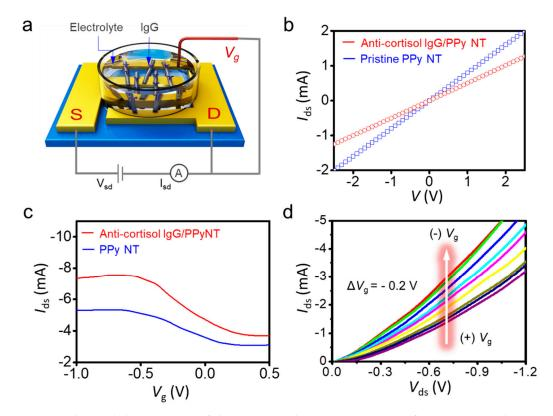
**Figure 3.** Electrical characteristics of the anti-cortisol IgG/PPyNT FET configuration. (a) Schematic representation of liquid-ion gated FET system (S: source; D: drain;  $V_g$ : gating voltage). (b) *I-V* values of before and after the conjugation of anti-cortisol IgG. (c) Transfer curves. (d) Source–drain current ( $I_{ds}$ )–bias voltage ( $V_{ds}$ ) curves from the anti-cortisol IgG FET configuration, with various gate voltages from 0.4 to -1.2 V.
