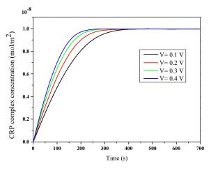
Figure 5. Effect of various voltages on the C-reactive protein (CRP) binding reaction.
