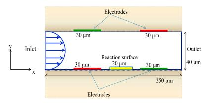
Figure 1. Schematic model geometry of the microchannel of the biosensor.
