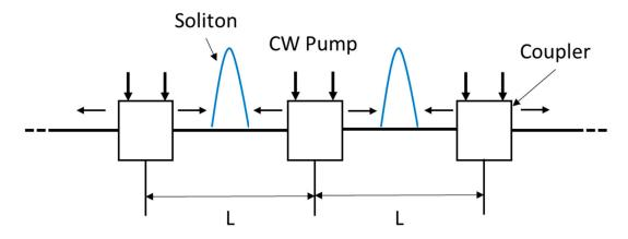
**Figure 9.** Schematic illustration of a soliton communication system. Solitons are amplified through SRS by injecting continuous wave (CW) pump radiation periodically.
