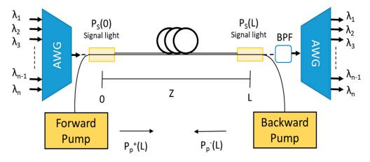
**Figure 3.** Schematic representation of multiplexing/demultiplexing based distributed optical Raman amplifier.
