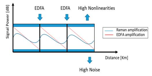
**Figure 4.** Ideal distributed amplifier: the loss is counterbalanced at every point along the span, leading to an improvement of the signal to noise ratio (SNR) respect to (ideal) discrete amplification.
