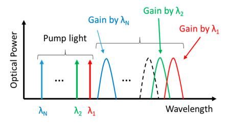
Figure 6. Multi-wavelength pumping technique for wideband Raman amplifiers.
