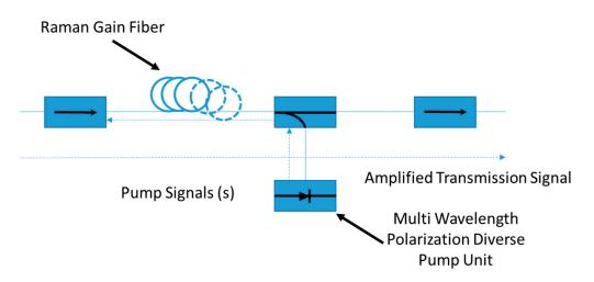
Figure 5. Discrete fiber Raman amplifier (FRA) scheme with pump power confined to the lumped element.
