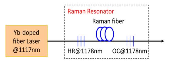
**Figure 7.** Schematic representation of a Raman fiber laser with one wavelength shift. (HR—high-reflectivity fiber Bragg grating, OC—output coupler—a low-reflectivity fiber Bragg grating).
