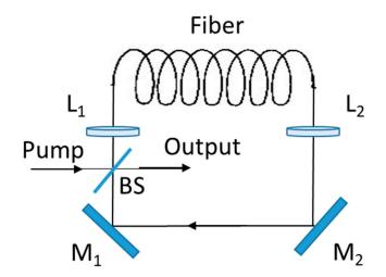
**Figure 10.** Schematic representation of the ring-cavity geometry implemented for Raman soliton lasers. BS is a dichroic beamsplitter,  $M_1$  and  $M_2$  are mirrors of 100% reflectivity,  $L_1$  and  $L_2$  are microscope objective lenses.
