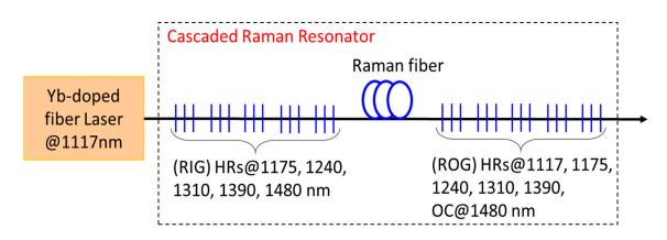
**Figure 8.** Schematic representation of a Raman fiber laser with multiple wavelength shifts by using a cascaded Raman resonator (RIG—Raman input grating set, ROG—Raman output grating set).
