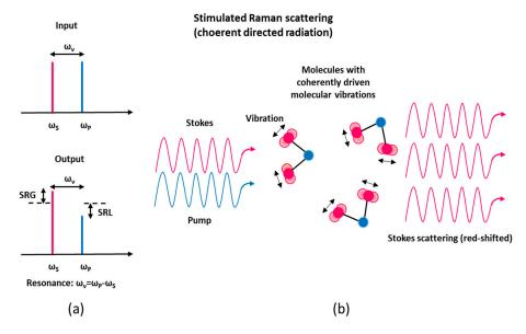
**Figure 1.** Stimulated Raman-Scattering (SRS) principle. (**a**) Pump–probe modalities associated with the SRS process are pointed out: SRG, stimulated Raman gain; SRL, stimulated Raman loss. (**b**) Stimulated Raman scattering occurs through inelastic scattering of probe photons off from vibrationally excited molecules that interfere coherently.
