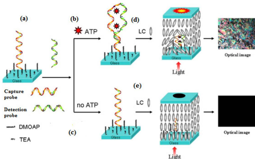
**Figure 10.** Stepwise assembly of the LC biosensing substrate based on ATP aptamer. (1) immobilization of capture DNA probe on the TEA/ DMOAP mixed SAM modified glass slide (a); (2) hybridization with detection DNA in the presence of ATP (b) or in the absence of ATP (c); (3) The corresponding 5CB LC cells (d,e) fabricated with the DMOAP-coated glass slides (upper) and the modified slides (b,c; lower) [31].
