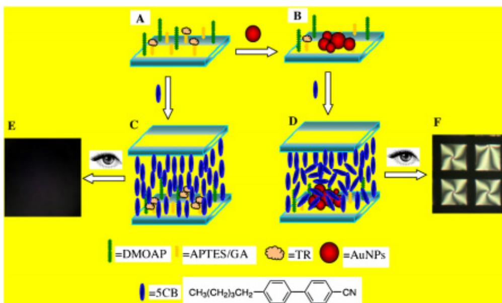
**Figure 9.** Illustration diagram of detection strategy of LC biosensor: (A) immobilization of TR; (B) deposition of AuNPs through the enzymatic process; (C) homeotropic orientation of 5CB in the cells without AuNPs on glass slides; (D) the disrupted orientation of 5CB in the cells with AuNPs deposited on glass slides. Photograph under polarized light microscope (E,F) [30].
