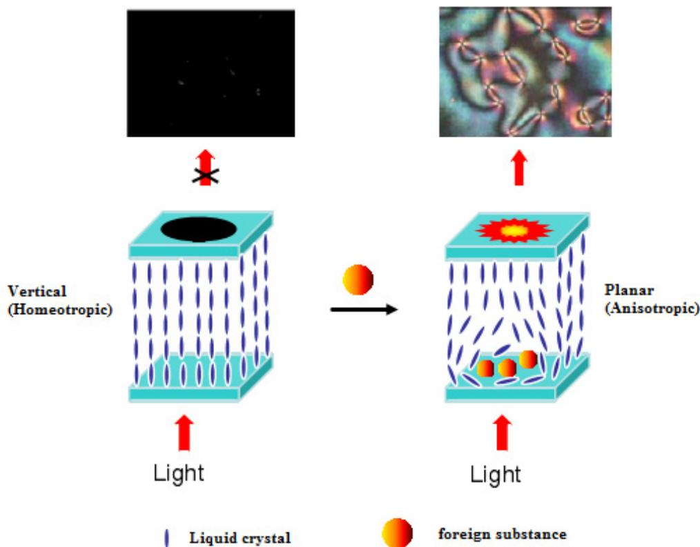
Figure 1. Schematic diagram of liquid crystal biosensor detection.
