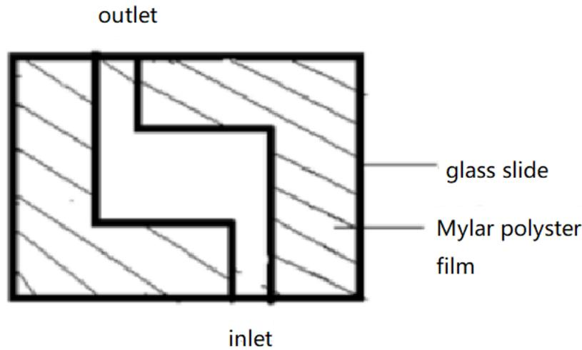
Figure 3. ‘L’-shaped cell for LC–solid interface sensing.
