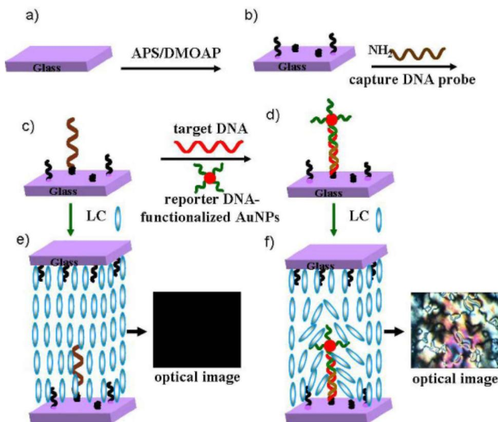
**Figure 7.** Principle of of LC biosensor based on gold nanoparticles signal enhancement. (a) cleaned glass slide; (b) assembled APS/DMOAP substrate; (c) fixed capture DNA probe substrate; (d) occurrence of binding events; (e) optical image of LC sensing cell before binding events; (f) optical image of LC sensing cell after binding events, disruption of the homeotropic LCs [28].
