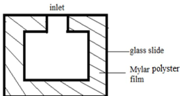
Figure 2. Cell for LC–solid interface sensing.
