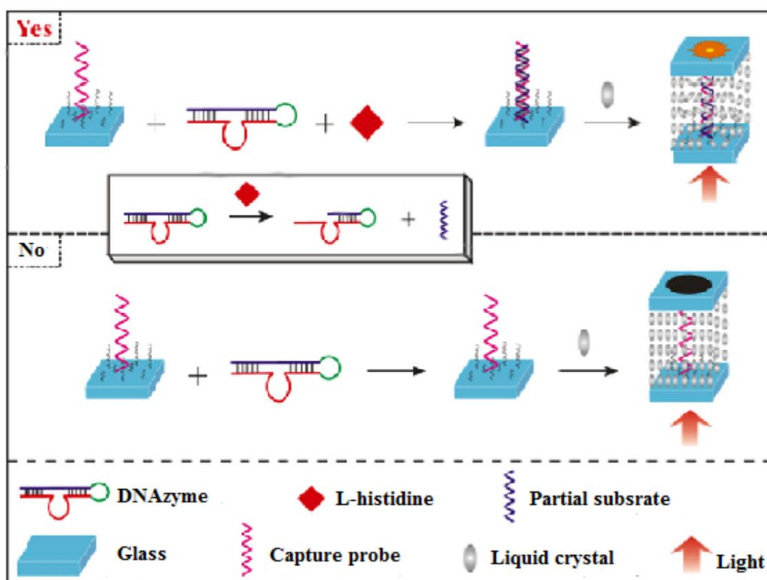
**Figure 11.** Description of the high-sensitivity DNAzyme-based LC biosensor for L-histidine. Only L-histidine can cleave the DNAzyme and release partial substrate, which hybridizes with the capture probe forming ds-DNA on the glass slide. The ds-DNA induces a homeotropic-to-tilted transition of the LCs, resulting in a birefringent texture of the optical image for LC cell [32].
