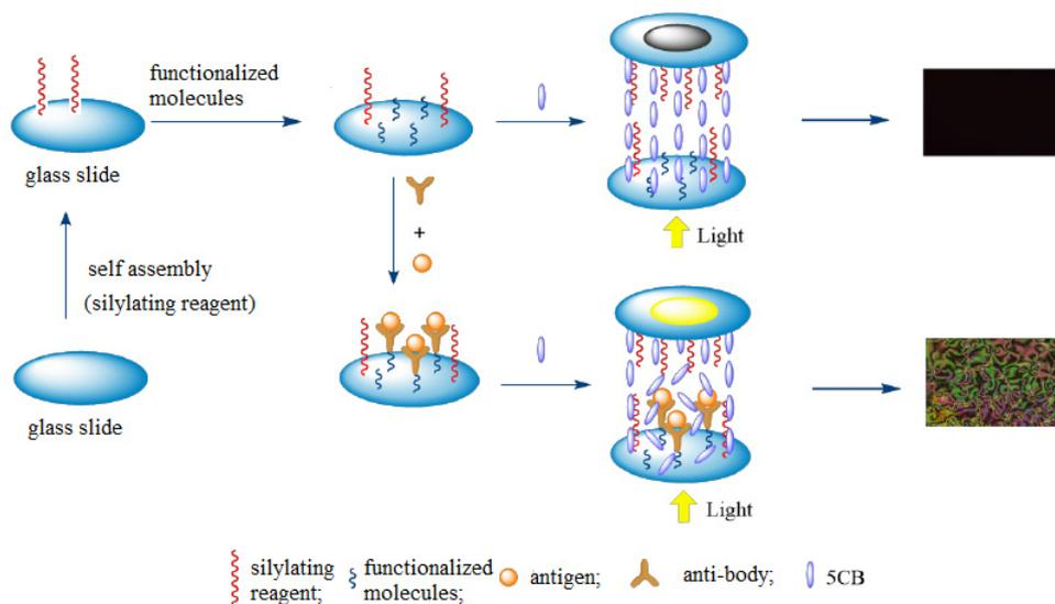
Figure 4. Diagram of the LC–solid interface sensing principle.
