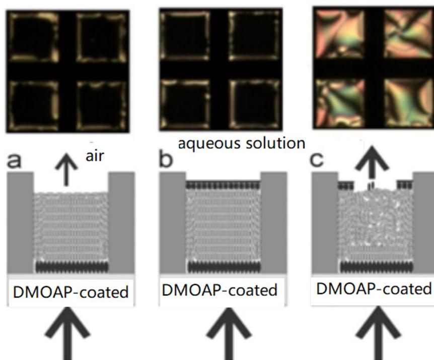
**Figure 5.** Schematic representation of an LC-based sensor consisting of a gold grid compartment, a silanized glass substrate and LCs; the arrows indicate the transmission of light: (a) LCs appear aligned near the substrate and slightly disordered near the air interface. (b) LCs exhibit homeotropic alignment near an aqueous environment, mediated by a lipid layer. (c) Destruction of the lipid layer results in disorder of the LCs [6].
