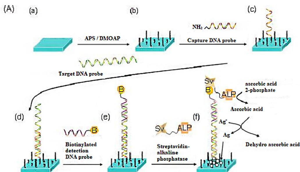
**Figure 8.** Stepwise assembly of the signal-enhanced LC DNA biosensing substrate based on enzymatic silver deposition: (a) cleaned glass slide; (b) self-assembled APS/DMOAP film; (c) immobilization of capture DNA Probe; (d) hybridization with target DNA; (e) hybridization with biotinylated detection DNA probe; (f) association with streptavidin alkaline phosphatase and reduction of silver ions by ascorbic acid [29].
