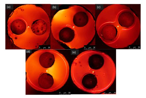
**Figure 1.** Second harmonic (SH) micrographs of twin-hole silica fibers poled in different electrical configurations, namely (a) conventional anode–cathode, (b) single anode, (c) anode–anode, (d) single cathode and (e) cathode–cathode. The figures are extracted from the work of An et al. [38].
