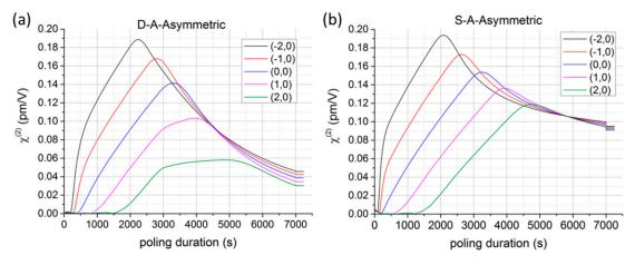
**Figure 7.** Time evolutions of the  $\chi_{eff}^{(2)}$  numerically obtained for a twin-hole fiber of asymmetric geometry poled in (a) D-A and (b) S-A configurations. The values of  $\chi_{eff}^{(2)}$  have been calculated via Equation (3) at five different locations in the fiber's core region (4  $\mu$ m diameter) and in the plane Y = 0. The legend shows the (x,y) coordinates (in  $\mu$ m) of the points where the values of  $\chi_{eff}^{(2)}$  have been calculated [45].
