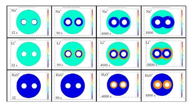
**Figure 2.** Temporal evolution of the mobile cations for a Germania doped twin-hole fused silica fiber poled in a cathode-less configuration (the two electrodes inserted in the two cladding channels are connected to the same potential of 5 kV). The injection of the  $H_3O^+$  ions is considered inexhaustible and capable to neutralize the non-bridging oxygen (NBO $^-$ ) centres depleted of the impurity positive ions moved because of the application of the external electric field [39].
