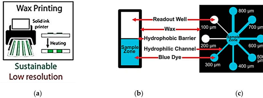
**Figure 2.** (a) Wax patterning on a paper substrate, followed by heating step, to create hydrophobic borders across the substrate. (b) A typical example of a  $\mu$ PAD device for the minimum hydrophobic barrier test. Black boundaries show printed wax which prevents liquid to flow out of channel. (c) A paper-based device with multichannel system of various widths (adapted with the permission from Creative Commons Attribution-Non Commercial-No Derivatives License) [17].
