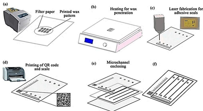
**Figure 11.** Schematic of the microchannel fabrication and microchannel enclosing using wax printing and laser cutter where (a) printing wax pattern on a filter paper, (b) heating step to penetrate wax through paper, (c) laser fabrication for adhesive seals, (d) inkjet printing of QR code and scale (e) enclosing microchannels by combining device layers, and (f) final device construct. (Adapted with the permission from Springer Nature) [68].
