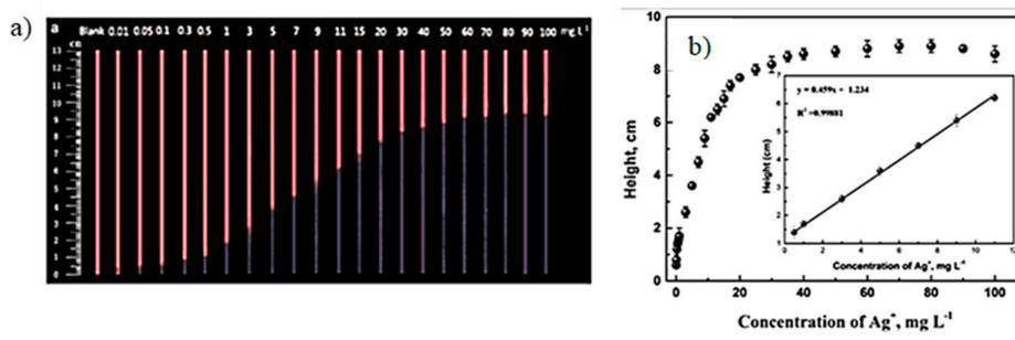
**Figure 7.** (a) Quenching of the fluorescence band in the presence of different concentrations of  $\text{Ag}^+$  in mg/L under UV light at 365 nm. (b) Corresponding calibration curve obtained in the presence of various concentrations of  $\text{Ag}^+$ . (Adapted with permission from American Chemical Society) [45].
