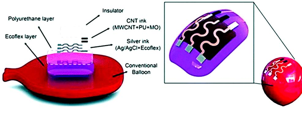
**Figure 3.** An example of wearable sensor demonstrated on a balloon which shows adaptability to curvilinear surfaces. The multiple layers consist of an Ecoflex layer (inner), polyurethane (intermediate), a printable sensor (Ag/AgCl with Ecoflex composite) and a flexible insulator layer (upper) (Adapted with the permission from Wiley Materials) [18].
