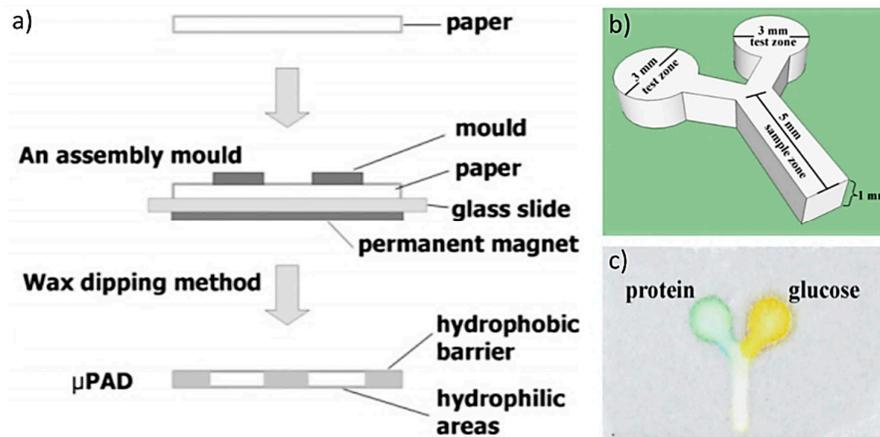
**Figure 5.** Wax dipping method and detection of analytes: (a) Procedure for patterning paper by wax dipping (left). (b) Shape and size of an iron mask. (c) Detection of protein and glucose on a paper microfluidic device by the wax dipping method (Adapted with the permission from Elsevier) [29].
