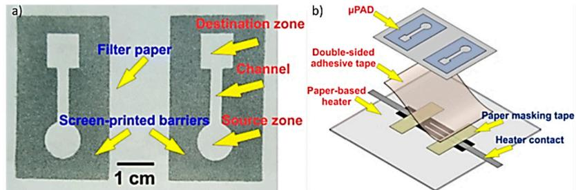
**Figure 12.** (a) Image of paper-based  $\mu\text{PAD}$ , which is fabricated by screen-printing of crayon eye liner on filter paper. (b) Schematic shows the process of sticking the  $\mu\text{PAD}$  to the paper-based heater using a piece of double-sided adhesive tape (Adapted with the permission of Springer Nature) [69].
