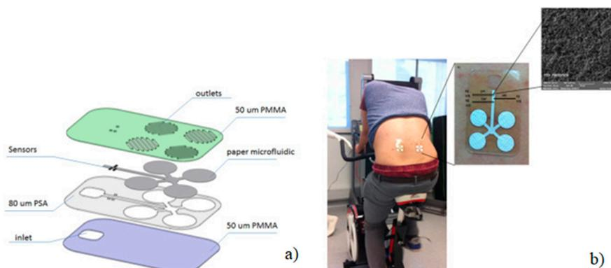
**Figure 13.** Schematic representation of the fabrication steps of the micro-fluidic chip on PMMA where (a) device layers, assembly and application on human sweat monitoring and (b) sensor structure and surface (Adapted with the permission of Elsevier) [71].
